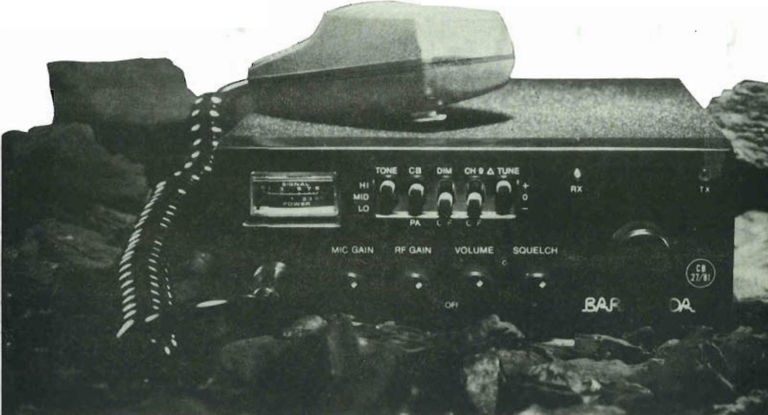
From the results in the table, we can see the frequency response is good but the modulation level at maximum (200 m/v) is 30% below the allowed level thus resulting in low modulation.
