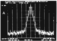
Spectral purity of the synthesizer from a spectrum analyzer.
