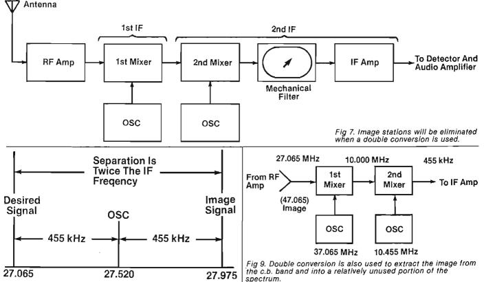
Fig 8. The relationship between oscillator, desired and image signals.
