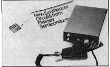
WR Electrotechs prototype c.b. stands proud from the Sanyo 7131 circuit notes (The LC 7131 is the chip used in the majority of FCC/CEPT sets).
