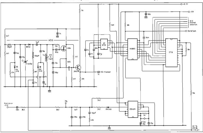
Fig 1. Single-loop synthesizer circuit diagram. Main elements are: the v.c.o. (left), reference oscillator (bottom), the SP8793 dual-modulus divider, the NJ8812 synthesizer controller and the 2716 r.o.m. i.c.
