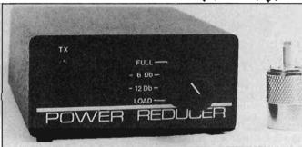
marked LOAD. This enables a transmitter to be keyed with the antenna removed, for test purposes without damaging the P.A. With an input of 4 watts, 1 watt and <sup>1</sup>/<sub>4</sub> watt.
