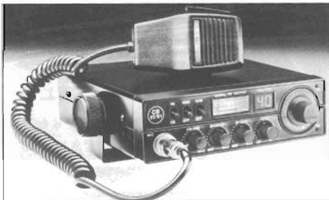
The LCL upmarket set, known as the 'Communicator' has logic synthesizer circuitry.
