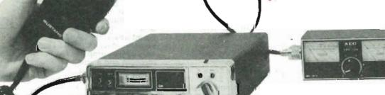
The SWR meter is fitted between the rig and antenna with a patch lead
