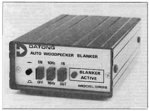
blanker removes any remaining clicks from the loudspeaker. The SRB2 connects in series with the antenna and loudspeaker terminals and internal modifications are not required.
