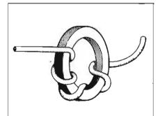
Figure 2. Winding each end of TV coax through a ferrite ring. Make as many turns as possible.
