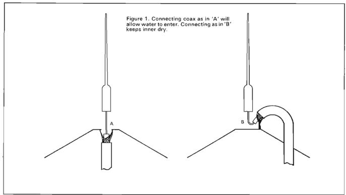
magnificent conductor the same effect will occur, even in good quality coax, if damp has been allowed to permeate it. To prevent this from happening it is advisable to join the cable to the antenna in such a way as to prevent water flowing from the antenna getting inside it. See Figure 1.
