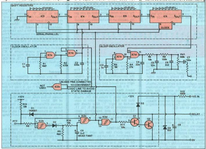
Fig 2: The circuit diagram showing all the components
