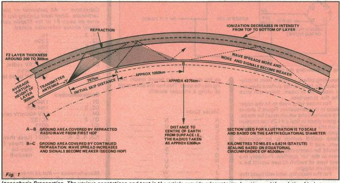
Ionospheric Propagation. The various annotations and text in the article provide adequate explanation and the relationship between critical frequency and usable frequency. Diagram is to scale i.e., virtual height of F2 layer relative to equatorial circumference of the earth.
