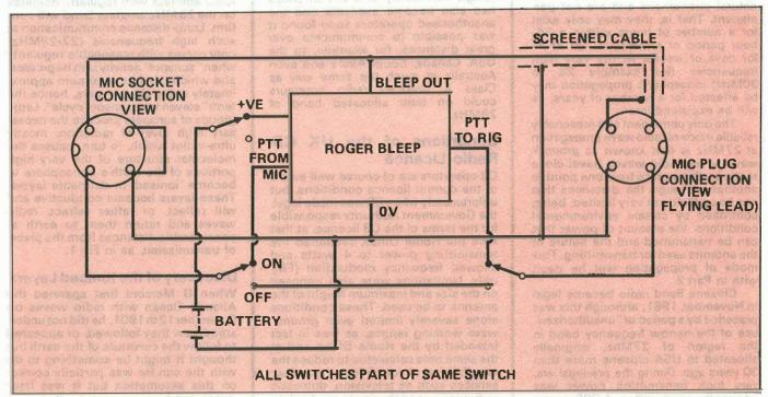
Fig 6: Connections used if the unit is to be cased separately
