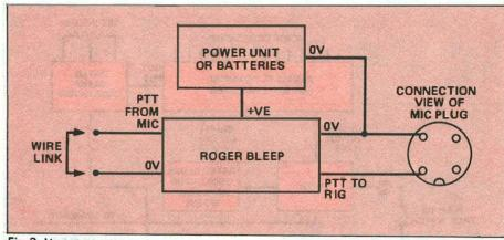
Fig 3: How to connect
