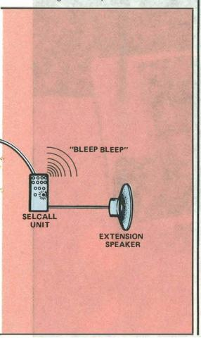
the set to remain 'asleep' whilst turned on with its receive amplifier muted until the correct code out of the 160 is received. The amp is released and a warble sounds through the loudspeaker or PA horn if fitted.
