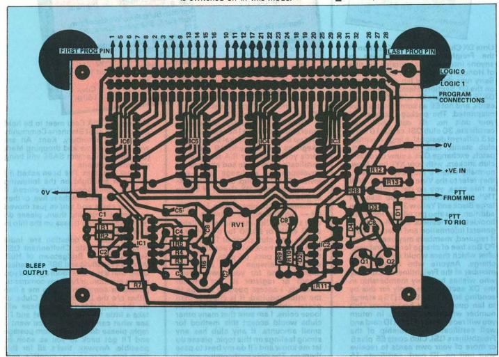
PCB and component assembly (seen from above — the tracks are on the other side of the board) The Small Deliberation above — the tracks are on the other side of the board)
