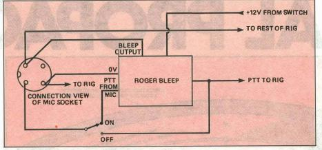
Fig 5: Connecting the unit to a rig
