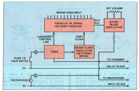
Fig 1: The circuit divided into its main parts
