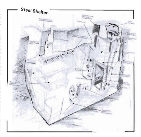
Basic design of a steel shelter made in Chesterfield by Newbridge Fabrications Ltd. The manufacturers recently ran a trial with a family. The main complaint from the family was that they were unable to make tea (in wartime there'd be no elec-
