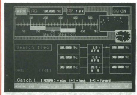
The AR2001 screen display on a home computer. The basic program runs lots of sub-routines that handle scanning; memos and search facilities. This is from the prototype board — so some the the display is in Japanese.
