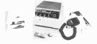
When you buy a new mobile transceiver today, you usually get a mounting bracket, a microphone that matches the transceiver, a microphone hanger, mounting hardware, fuses, mounting instructions, owner manual, and warranty card.
