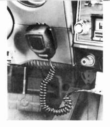
Install the microphone hangup bracket near enough to the transceiver that the cord doesn't stretch. And of course hang the mike so you can reach it easily from driving position. You'll find a dozen good places in almost any car, all of which meet these two criteria.
