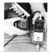
With Squelch open and the car engine running, you'll probably hear a lot of popping noise. In cars with high-energy ignition systems, this interference can really disturb communications.
