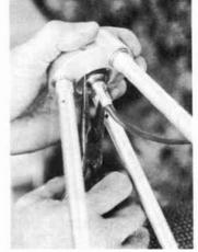
Place the insulator hub on the ground, with the tripod of radials pointing upward. If it's convenient, lean the radials against a shed, fence, or garage or house wall. Bring the end of the antenna mast near the hub, so the cable connector can be screwed onto the connector receptacle in the bottom side of the hub (facing upward right now). Tighten the connector with a pair of longnose pliers. (That's the only tool that reaches the connector to tighten it in these close quarters.)
