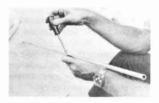
Select the "longest" end of the 24-inch tube—where the drilled hole is 3 inches or so from the end. Slip that end of the 24-inch tube into the drilled end of the 51-inch tube. Align the holes, and lock the tubes together with two of the self-tapping screws.
