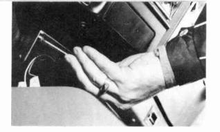
We chose a Cobra model 21 for our sample installation. Its size, in this instance, allowed us to mount it right over the center console in this 1975 Cutlass. Principles are the same for other CB radios and other cars.
