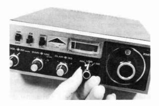
To take advantage of single-sideband, use only ssb transceivers in your personal system. Use upper- or lower-sideband modes during your working hours, when you need peak efficiency. You can join neighborhood gab sessions at night by switching to the a-m mode.
