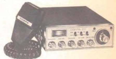
*This Cobra 29 mobile rig has a front panel mike gain control. (Dynascan)*
