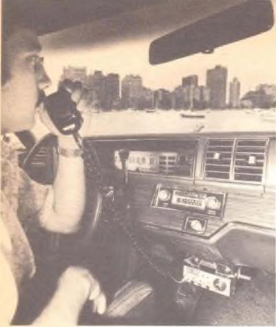
*A slide mount as used on this Cobra offers the advantage of quick removal for security. It's also a necessity if the same radio is to be used as a base station or changed frequently from one car to another.*
