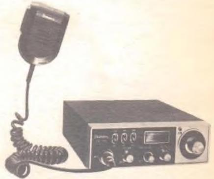
The Model CB-755 from Boman has a meter circuit to make SWR measurements.
