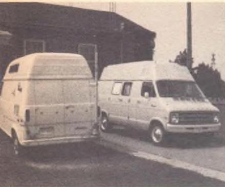
Two FCC mobile units, used to locate illegal transmitters.
