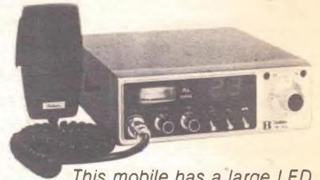
*This mobile has a large LED readout for channel indication and can be used with a telephone handset instead of microphone and speaker. (Boman Industries)*
