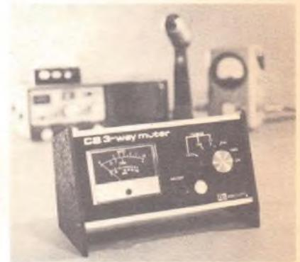
Antenna standing wave ratio meters come in a variety of shapes and sizes. Antenna Specialists' M-272 measures absolute power output as well as reflected power and modulation percentage.
