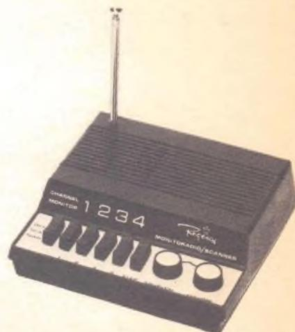
*Eavesdropping on police, fire or other VHF/FM services is the current SWL rage. Regency's ACT-C4 is a 4-channel scanner that covers both VHF high and low bands along with UHF.*
