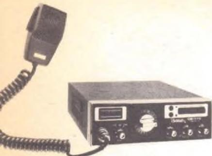
*Boman Model CB-770 is a mobile capable of SSB and AM operation.*
