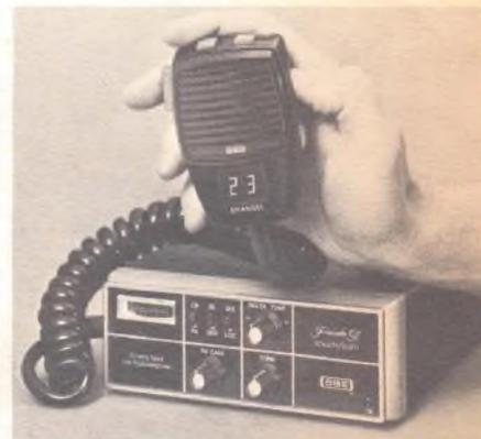
*Though it looks fairly conventional, all the primary operating controls including volume, squelch, channel selection and LED readout are mounted on the microphone of SBE's Model 32 CB.*
