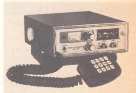
Many hams still build their own equipment though much of what they build today comes from kits. This is Heathkit's Model HW-2036 synthesized 144 MHz transceiver. Note the Touchtone® pad mounted on the microphone, which enables the user to dial up his own telephone number through an appropriately equipped repeater.
