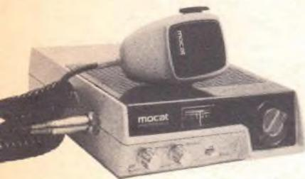
Current mobile rigs are more compact and designed to fit in with a modern auto's decor. This Motorola Mocat is designed for under-dash mounting.
