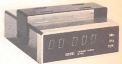
*A frequency counter is a must for checking transmitter frequency accuracy and stability. This BOHSEI is usable to 30 MHz.*
