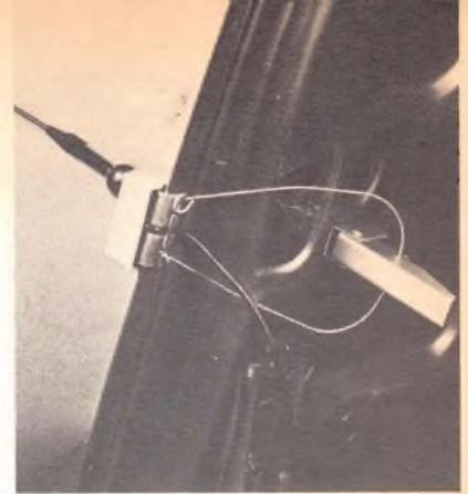
*The spring-loaded latch of this lip-mounted antenna permits its release in an instant for trunk storage while the user's car is parked. (South Com)*
