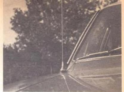
A disguise antenna has no loading coil so looks exactly like the BC antenna in whose mounting hole it fits. This helps avoid tipping rip-off artists that the car is CB-equipped. A special coupler lets it operate on both CB and the broadcast band. (Antenna Specialists)
