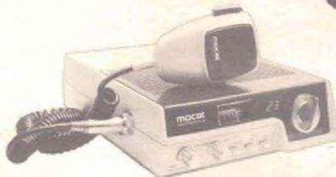
*Motorola Mocat Model 2020 features an LED channel indicator and noise blanker.*
