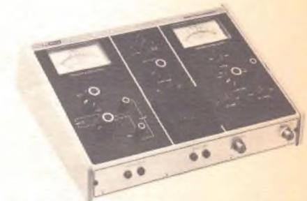
*One of the more ingenious CB service ideas to come along is B&K's 1040 Servicemaster. With the addition of only a signal generator, it checks out all of a CB set's operating parameters.*
