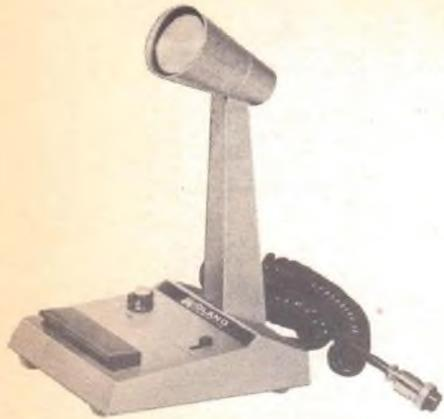
Accessory base station mikes offer more features than those usually supplied as original equipment and are almost a must when a mobile rig is used as a base station. This example from Midland has a locking push-to-talk switch and built-in pre-amplifier.
