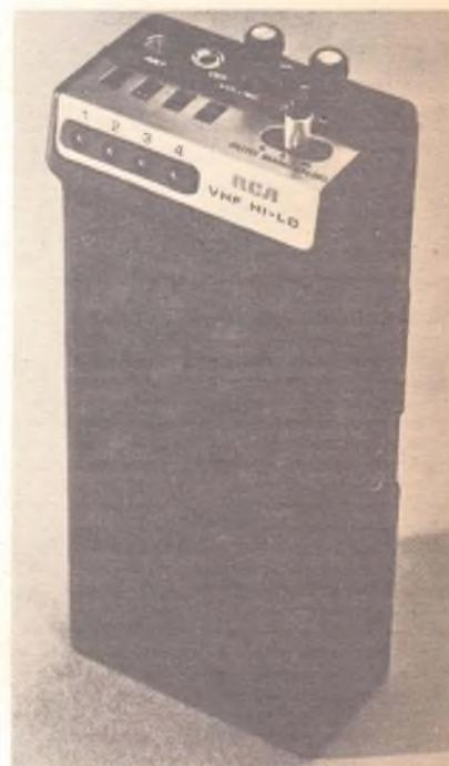
*Pocket scanning receivers are also available in sizes little larger than a cigarette package. The RCA 16S100 is a 4-channel scanner that can monitor a combination of VHF and UHF frequencies.*
