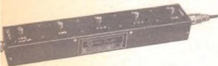
Use of a low-pass filter keeps harmonic of your transmitter's output signal from getting to your antenna and being radiated into nearby TV and FM receivers. This Telco Products' model can be tuned for minimum interference to a specific channel.
