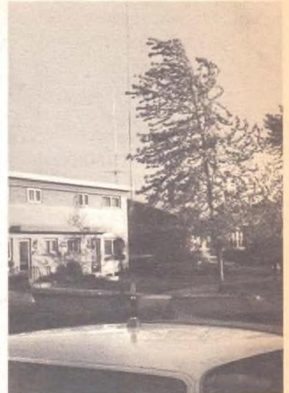
*A rooftop installation is the neatest appearing, most uniform in radiation and toughest to install of all mobile antennas.*
