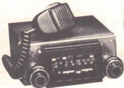
Tenna's A1301 is an in-dash combination 23-channel CB and AM/FM stereo receiver.
