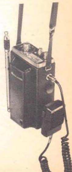
*Another approach to portable operation is an accessory battery pack powered mobile rig like this. (Midland International)*
