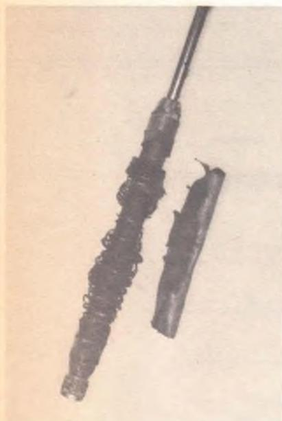
You don't have to be high to get hit by lightning. This loading coil was on an antenna mounted on the roof of a mobile home.
