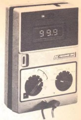
Digital multimeters like this B&K Model 280 are much more precise and easier to use than conventional VOMs and still retail for under \$100.
