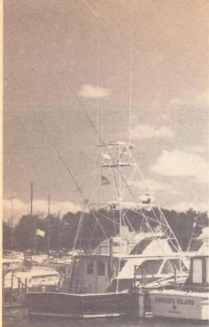
*This sports fishing boat carries antennas for low frequency SSB, VHF/FM and CB communications plus radar.*
