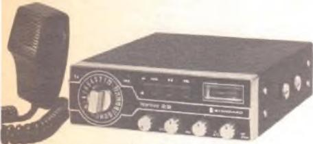
The more elaborate mobile rigs like this Horizon 29 also boast an impressive number of controls. (Standard Radio)
