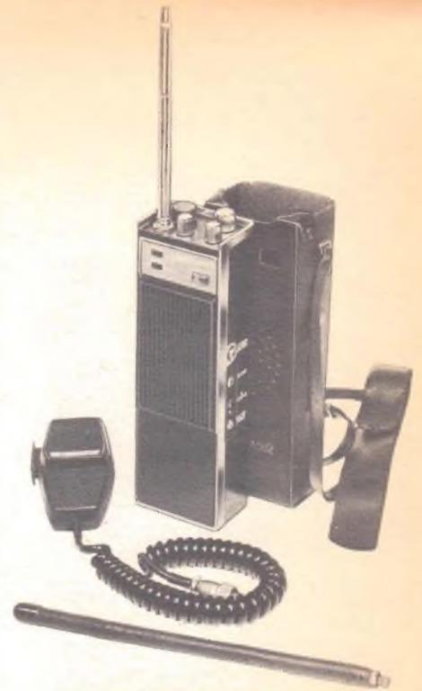
*Midland's 5-watt, 6-channel transceiver can be used with a speaker/microphone, features a jack for an external antenna and top-mounted controls. Note optional flexible "rubber ducky" antenna.*
