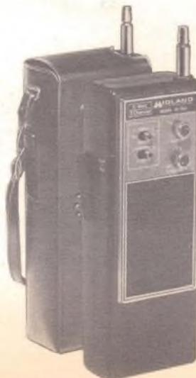
100-milliwatt transceivers are primarily very short range units, transmitting up to a mile line of sight but much shorter distances in heavy brush.
