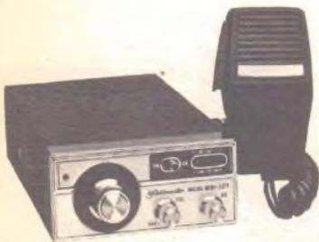
*This very compact unit has a row of LED lamps instead of a meter for signal strength and output indication. (Fieldmaster)*
