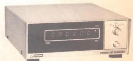
*This six digit frequency counter from B&K signals the user if a frequency beyond its 100 MHz capability is applied.*
