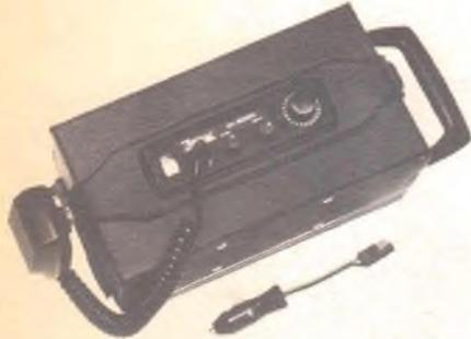
Transcom assembles different manufacturers' equipment into a variety of portable packages. This one includes two large speakers and an automatic polarity inverter for positive ground cars with a Zodiac M-5023 CB set.
