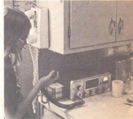
*Base station CB installations offer many more options and much fewer problems than their mobile counterparts. Putting the station in the kitchen placed it near the center of activity, convenient to both telephone and windows for antenna lead-ins.*
