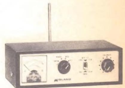
This Midland antenna standing wave ratio meter can also double as an antenna field strength meter using the telescoping antenna mounted on its rear panel.
