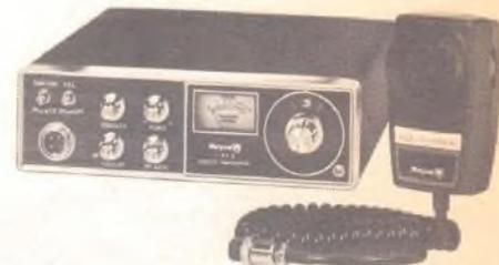
*Royce Model 1-658 mobile rig. Note the gain control built into the microphone case.*
