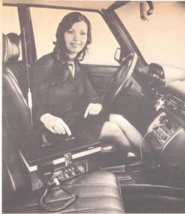
Greater user convenience is provided by a portable package such as this one by Kris. With front panel, speaker grill and antenna accessible without opening the case, it need only be plugged into a power source to go on the air.
