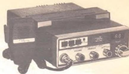
*An LED channel indicator highlights the Regency Model MT-55 synthesized marine radio which covers all 55 domestic and international marine FM channels.*
