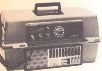
*If your boat is harbored in an area where break-ins are common, you'd be wise to consider one of Trans-Comm's portable packages. The M-2940 combines a Royce VHF marine transceiver and a Regency Whammo-10 programmable VHF scanning receiver.*
