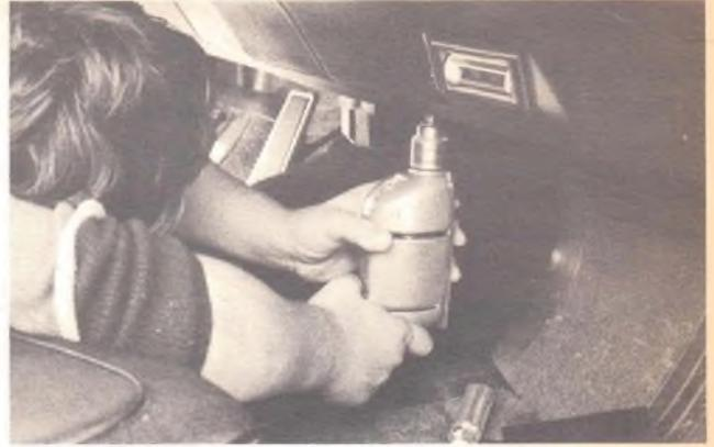
*Use the mounting bracket to locate the mounting bolt holes, then drill the holes taking care not to damage car wiring or accessories behind the dash with the drill bit.*
