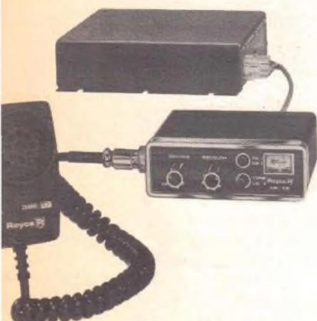
*Royce's remote mount radio has channel selection and indication on the microphone, other controls on the control head.*
