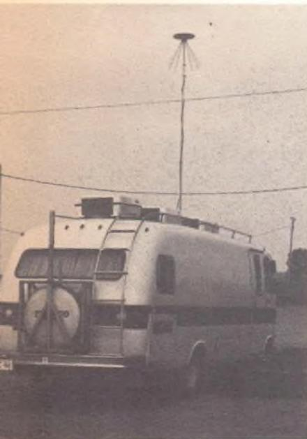
Another FCC mobile monitoring unit, this one used to compile spectrum occupancy data.
