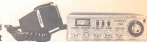
*Cobra 138 from Dynascan is an SSB as well as AM transceiver.*
