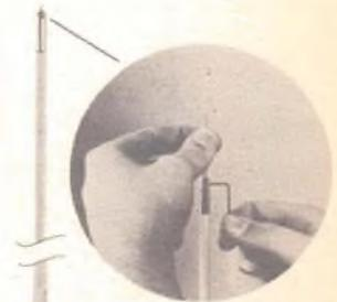
Tunable top-loaded antennas (left) usually have a short stub for adjustment. (Avanti)
