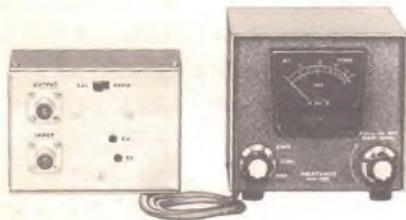
Antenna meters like this Heathkit HM-102 are designed to be left in the antenna circuit continuously so have their indicator portion separate from the detector.
