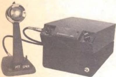
Here's a mobile radio being used as a base with a desk type mike and auxiliary AC power supply. (Standard Communications)
