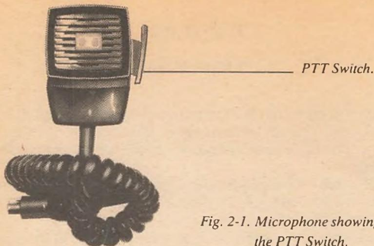
*Fig. 2-1. Microphone showing the PTT Switch.*
