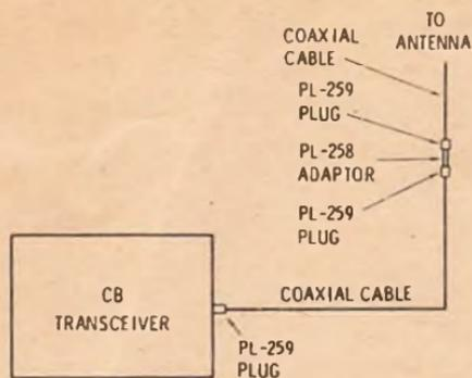
*Fig. 6-5. Use a PL-258 Adaptor when extending coaxial cable.*
