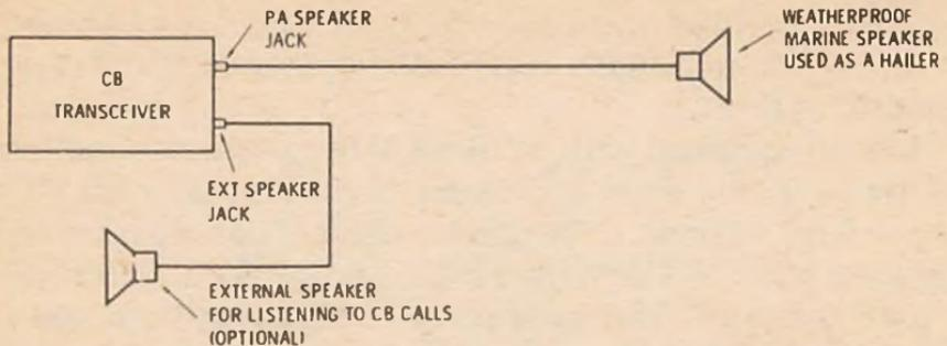
*Fig. 6-2. Hook-up of a "Hailer" Speaker.*
