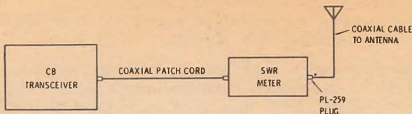
*Fig. 4-4. Hookup of SWR Meter for Testing Antenna.*
