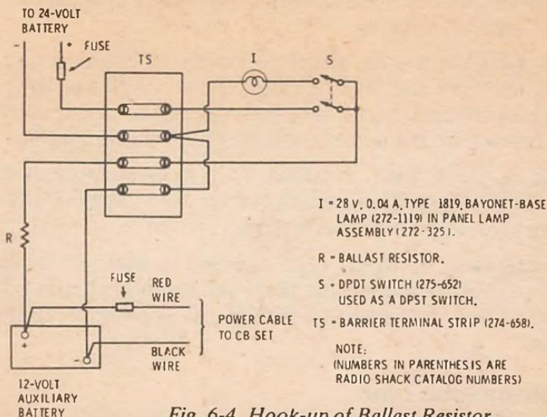
*Fig. 6-4. Hook-up of Ballast Resistor and Charging Control.*
