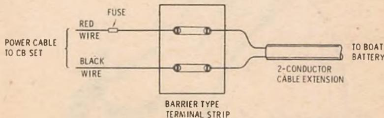
Fig. 6-3. Extending the Power Cable.
