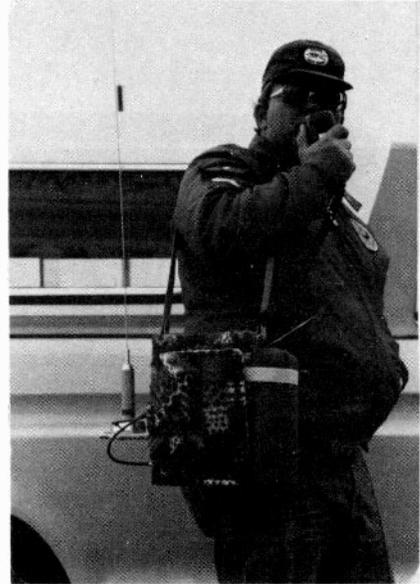
"The Box" has a unique lid that doubles as a pocket for excess antenna wire or carrying misc. items. Radios are mounted in "The Box" by special shock foam, giving the S.B. 360° ventilation and protecting it from road vibrations, hard knocks, etc. Installation requires a sharp knife and takes approximately 5 min. Accessories for "The Box" are a 12 Volt battery pack and antenna (magnetic) mount.
