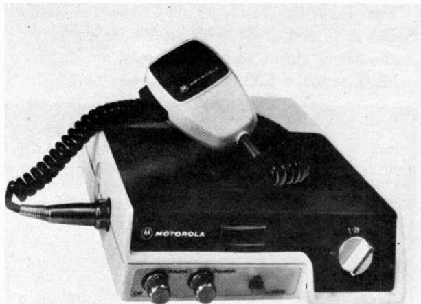
Motorola has unveiled a line of four U.S.-made under-dash 40-channel citizens band radio models. The basic unit, model 4000, offers such standard features as a digital phase lock loop synthesizer; a dual gate F.E.T. front end; a rugged plug-in Motorola power microphone with a built-in amplifier; a top fire speaker; a large, illuminated S/R/F meter; an automatic noise limiter and a wide range automatic gain control.
