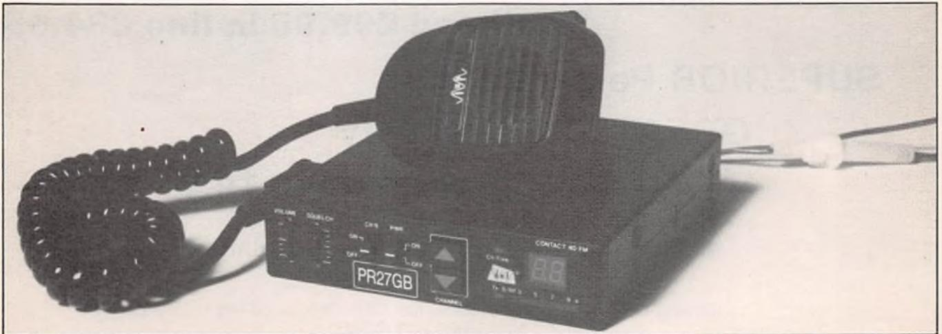
The only other point is that the volume and squelch controls are a little fiddly to operate, particularly whilst mobile over less than perfect roads. The short travel makes fine adjustment awkward and although somewhat a matter of personal preference, I feel two conventional rotary controls here would be a lot better
