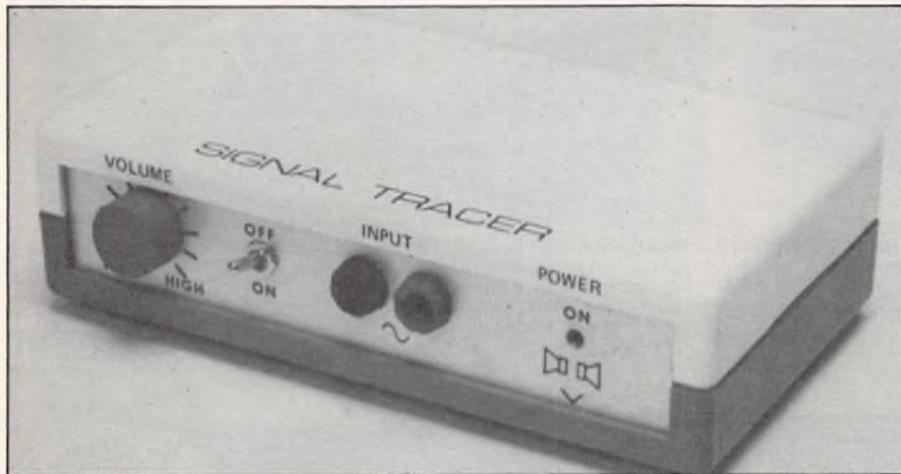
**T**his month's D.I.Y. project is that of a Signal Tracer; the natural counterpart of last month's project entitled Signal Injector. The tracer makes very light work of troubleshooting audio circuits (such as that no-good microphone!) as bad joints and faulty components are easily identified. The system is, very simply, a small audio amplifier which is battery-operated and it can report signals which may be but a few millivolts in amplitude.
