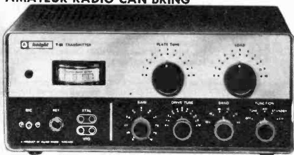
**T-60 6-Band 60-Watt Peak AM/CW Transmitter Kit**
