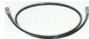
Prefabricated N to N cables cost less than your labor and materials. Allied jumper cables feature RG-213U coaxial cable, N-Male connectors with shrink-tube weatherproofing. Special lengths available on request. 7.8 dB loss per 100 feet at 900 MHz.
