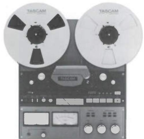
A 2-track 1/4" 2 channel half track mastering and broadcasting recorder/reproducer with 10 1/2" reel capacity, sync capability, full servo, SMPTE interlock capability through accessory connector and punch in/out recording. The 42 also features NAB or IEC equalization, dump edit, search to zero and search to cue, 7 1/2-15 ips speeds and +4/-10 input/output.
