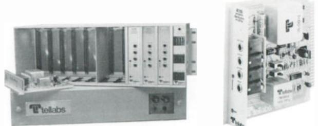
Each Tellabs 4018 module provides a 1 x 8 distribution amplifier with high impedance bridging or 600 ohms input and 600 ohms each port output. The 1012 housing permits mounting of up to eleven 4018 modules plus a 9021 fuse protection module. Combine this package with a rack-mounted 8013 power supply, and you have up to 11 x 88 distribution amplifier. All Tellabs equipment is connected by .075 wirewrap terminals. Cabinets must be wired by user.
