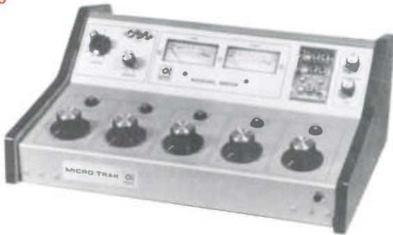
The Model 6509 audio console features five mixing channels, nine mixing inputs, outputs for stereo, mono, monitor, headsets and cue speaker, selectable muting, slotted screw terminal connections, illuminated VU meters. Crosstalk spec'd at -50 dB to -74 dB and distortion is 0.4% Re: +8 dBm output, 800 Hz, hi level input. Package size is 17 3/4 W x 12 3/4 D x 6 1/2 H and weighs 16 lbs.
