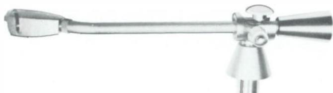
This attractive tone arm is constructed of tubular aluminum with a die-cast cartridge shell, that accepts all standard stereo or mono cartridges. It has a vertical height adjustment and friction-free chrome steel ball vertical movement. It tracks at 1 gram or less and includes a counterweight. Connects with standard plugs.
