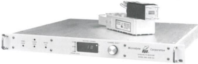
Looking for KU-Band? Allied has the most popular Microdyne 1100 BDC/DCR series! The first half of this receiver is the block down-converter (BDC) which converts the KU-Band frequencies, at the antenna, to a range of 270-770 MHz. Lower cost cable can then be utilized between the satellite antenna and the receiver. Also the BDC is available in a C-Band version which allows you to get double service from your DCR receiver!
