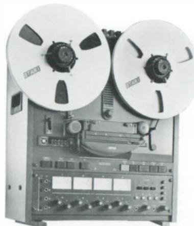
1/4" four channel, quarter track recorder/reproducer. DC-servo capstan with  $\pm 7\%$  vari-speed. 15-7 1/2 ips speed. +4 or -10 dB input/output level select. Real time tape counter with LED display. Zero return. Headphone output with channel select. Test oscillator (1 kHz or 10 kHz). Microprocessor controlled transport logic. Dynamic braking. Integral splicing block. External machine control interface connector for synchronizers.
