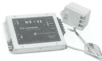
The ST-11 Pro-eminece phono pre-amp by Micro-Track is a super high performance unit. It is RFI resistant for use in AM, FM or TV. It is very compact and designed to match a 47K ohm magnetic stereo phono cartridge. Provision for a nominal 0 dBm output with headroom to a max. of +22 dBm. Distortion is .05 or less, THD and IM. The signal to noise ratio is -72 dB or better, also has a jumper selectable rumble filter internally.
