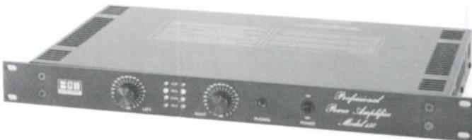
The BGW 150 is a rack mounted power amplifier rated at 50 watts per channel into 8 ohms, 150 watts into 8 ohms mono, with inter-modulation distortion of less than .02%, a frequency response of -.25 dB 20 Hz to 20 kHz and is designed for any load impedance equal to or greater than 4 ohms.
