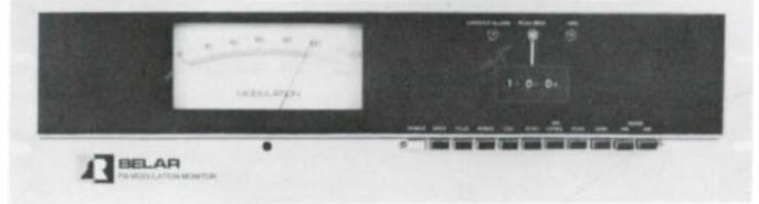
The FMM-2 sets new standards in accurate FM monitoring. It's the first to incorporate a sample hold peak modulation meter circuit independent of modulation polarity to allow the meter to respond to program peaks of the shortest duration. The heart of the FMM-2 is an ultra-linear digital discriminator which provides a distortionless baseband signal for accurate monitoring as well as precise stereophonic and SCA decoding.
