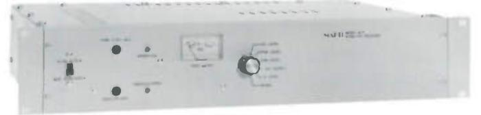
The Marti Studio-Transmitter Link/Intercity relay is a line-of-sight FM communications system providing a high quality broadcast audio channel with two optional sub-channels. A dual link for stereo provides two identical broadcast quality channels with better than 60 dB stereo cross talk and four optional sub-channels. This system offers greater rejection of interference, superior noise performance, low channel cross talk, greater redundancy, and lower cost.
