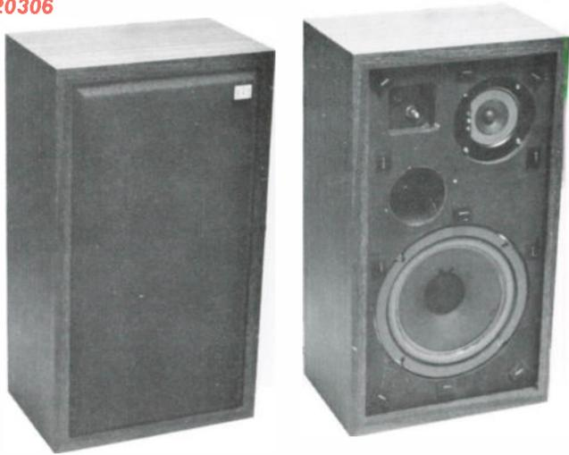
The MONITOR loudspeaker system provides a flat response from below 50 Hz to beyond 20 kHz. Its high compliance surround on the 8" woofer and phenolic tweeter combine to enhance any type of music. The tweeter control and the system fuse are behind the snap-away grille. It will handle 25 watts RMS continuous, 45 watts integrated program material at 8 ohms.
