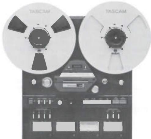
A 4-track 1/4" recorder/reproducer with 15-7 1/2 ips speeds, 10 1/2" reel capacity, full frequency response in sync mode, function and output select and punch in/out recording. The 34 also features ±12% pitch control, dump edit, cue control, FL tape counter and zero return.
