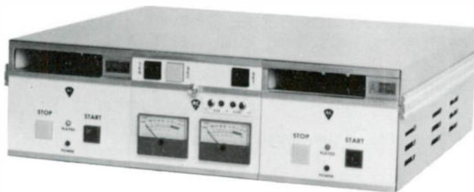
The Models E-50 through E-56 are dual transport record/playback machines which allow single deck or dual deck recording, sound on sound, composites and stereo to mono mix dubs. Features include a slide out front panel, interchangeable transports and other assemblies, 1 or 3 cue tones mono or stereo, a replay reminder system, full remote control that's automation compatible and latching connectors and slip/lift cover.
