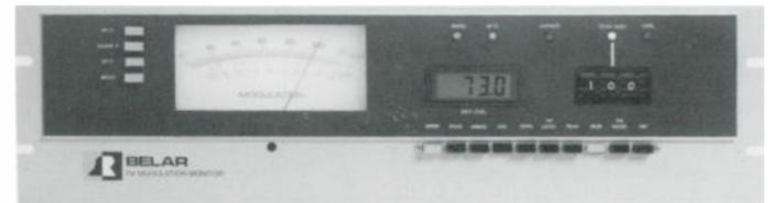
The Belar Model TVM-100 Television Aural Modulation Monitor is a precision wide band monitor designed to measure the total modulation characteristics of mono as well as multi-channel television audio. Utilizing split sound and quasi-parallel detection modes, automatic deviation calibrators for 25 KHz (mono) and 73 KHz (BTSC Stereo) and a digital display for indication of actual deviation, the TVM-100 satisfies all requirements for mono and stereo baseband monitoring and test.
