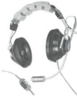
The CS-91 "Sportcaster II" is a professional sports announcer headset designed specifically for live, remote broadcasting. Omnidirectional dynamic boom microphone allows full freedom of head movement while the circumaural ear cushions screen out ambient noise.
