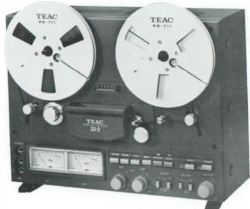
The basic half-track recorder/reproducer with independent record mode selector and 1 tape/source monitor for each channel. Independent mic/line mixing and output level control for each channel. Remote pause function for record and play. 7 1/2-15 ips speeds.
