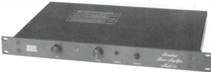
The BGW 85 is a rack-mounted power amplifier rated at 35 watts per channel at 8 ohms, with 0.1% T.H.D. 20 Hz to 20 kHz, 90 watts into 8 ohms mono, with 0.15% T.H.D. (The Model 85 features modular circuit assembly, toroidal mains transformer, packaged & cased transistors.
