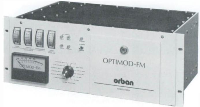
The ORBAN 8100A FM OPTIMOD® offers wideband or multiband operation, more versatile setup controls that permit precise "tuning" for different formats, improved voice/music balances, an improved stereo generator with cleaner baseband, new overshoot compensation that permits full modulation at all frequencies, yet doesn't increase low frequency IM distortion, plus a dual-chassis option, built-in crosstalk test generator, rigorous RFI shielding and true VC gain control. FM's favorite processor!
