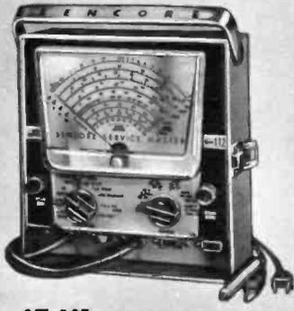
Two testers in one housing! Single test prod, 1% resistors, special scale indicators. 6" 200- $\mu$ a meter. AC-DC v.: 0-3-10-30-100-300-1000. P-P v.: 0-2800. Accuracy: DC,  $\pm$ 3%; AC,  $\pm$ 5%. Response (1st 4 ranges), 30 cps to 4.5 mc. Ohms: VTVM, 0-1000 megs, 6 ranges; VOM, 0-1 meg, 2 ranges. Inputs: VTVM, 10 megs; VOM, 5K/v. Zero center. 8<sup>1</sup>/<sub>2</sub>x7<sup>1</sup>/<sub>2</sub>x3<sup>1</sup>/<sub>2</sub>". With battery. For 110-120 v., 60 cy. AC. Shpg. wt., 6 lbs. Order Now.
