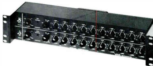
Each channel features 10 octave bands from 31.5 Hz through 16 kHz. ±10 dB control range. 12 dB/Octave high-pass filter variable from 20 Hz through 160 Hz. LED overload indicator. In addition an accessory socket provides for the insertion of optional low-level crossover networks. An EQ in/out switch is mounted on the front panel.
