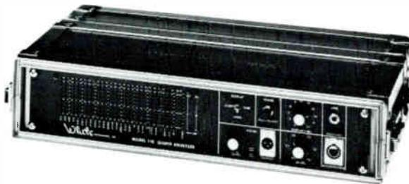
27 Double-tuned 1/3 octave filters on I.S.O. centers from 40 Hz through 16 kHz. 27 by 10 LED display plus separate dB-SPL and overrange readout. One and two dB scales. Display vernier. Built in pink noise generator. Mic and line level inputs. Sync and log amplifier outputs for remote oscilloscope display. Rugged road case. Meets ANSI S1.11-1971 Class II Specifications.
