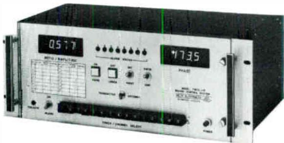
For AM directional arrays, complete transmitter and antenna monitor remote control capability can be found with the TMCS-1. This system works in conjunction with the Delta DAM-1 Digital Antenna Monitor to provide control and parameter display for both the antenna monitor, as well as the transmitter and associated equipment. The basic system provides 15 analog channel inputs, 8 alarm inputs, 15 on/off, raise/lower (cont.)
