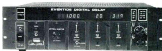
The modular construction of this unit makes it exceptionally flexible—up to five outputs, each with a maximum of 320 ms of delay (640 ms in the 'double' mode), selectable in 20 us steps. Optional modules available include a pitch changer, which will change the frequency of the input signal up to an octave above or below the original, and a remote control module which controls the delay line with a microcomputer.
