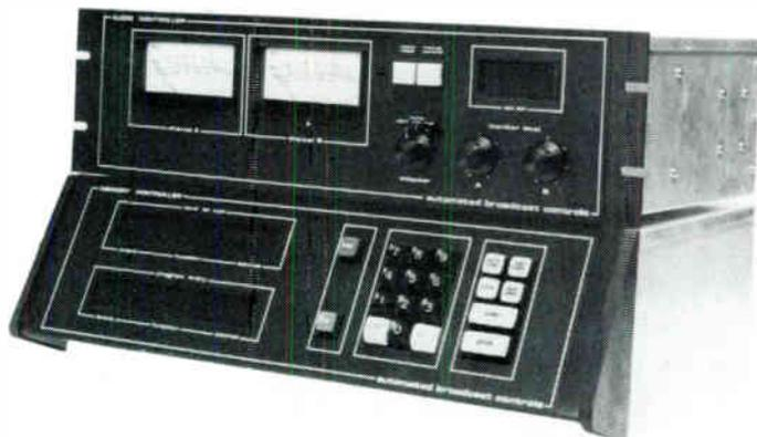
The new ABC 2800 APM Digital Automatic Program Control Center marks the introduction of ABC's FIRST generation automatic programming hardware. This completely random access audio switching system with solid state MOS memory storage and digital logic consists of three basic units.
