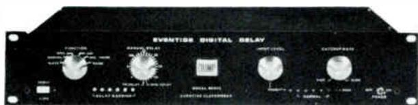
The BD955 was designed specifically for the policing of live talk shows. It is a RAM based digital delay line, available in two frequency ranges—7.5 kHz for reproduction of telephone audio, and 15 kHz for quality reproduction of the full audio spectrum. There are three maximum delay times available—1.6, 3.2 or 6.4 seconds.
