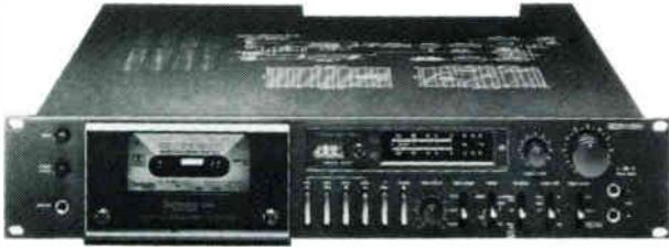
Behind its elegant "Flat-chassis" design, this cassette deck boasts a quartz-locked direct-drive capstan motor for durability and excellent speed control (wow and flutter is just 0.035% WRMS). Metal tape compatibility provides great specs: frequency response is 30-17,000Hz  $\pm$ 3dB with metal tape, and S/N ratio is 69dB.
