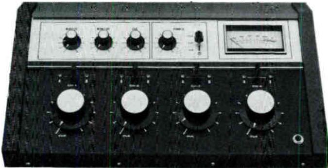
**COMPACT, PROFESSIONAL PERFORMANCE**—Incorporating modern solid-state technology, the Broadcast Electronics Model 4M50 4-Mixer Monaural Console affords professional performance at reasonable cost. Compact, yet uncluttered, the 4M50, with two inputs per mixer, can handle the selection and level control/mix of up to eight sources.
