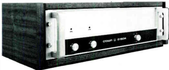
The CROWN D-150A is a single or dual channel power amplifier designed for precision amplification of frequencies from 1Hz to 20 kHz. The design of the D-150A provides extremely low harmonic and intermodulation distortion with very low noise. A switch on the rear of the unit allows stereo or mono operation with no internal wiring changes. In the mono mode, the D-150A is capable of a 50 volt balanced line output. The Unit operates on AC current from 120V to 240V.
