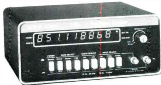
Bright's C1000 frequency counter is known throughout the communications industry for its ruggedness and reliability. This unit is housed in a tough .125" metal cabinet. Built to exacting commercial standards, many companies rely on the C1000 as their local frequency standard.
