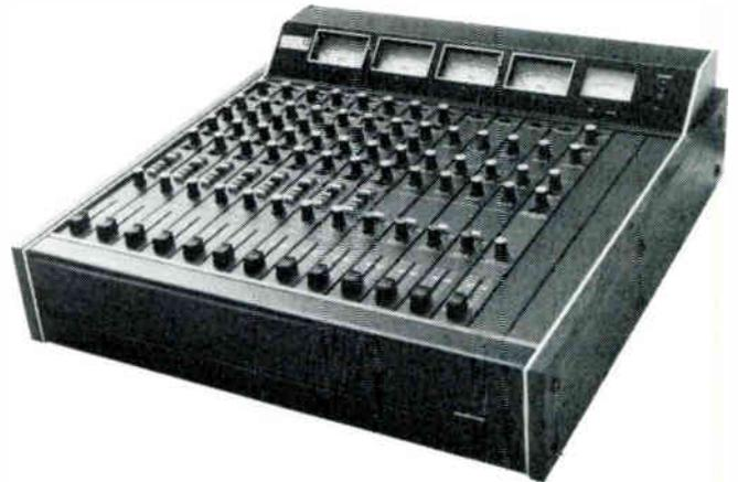
One of the hottest selling mixers available today is the Tascam Model 5. An incredible amount of control is packed into this small, sixty-two pound unit, and it has an amazingly low price tag. The basic mixer is modular, and has eight inputs and four outputs; an expander accessory can increase the total number of inputs to twenty.
