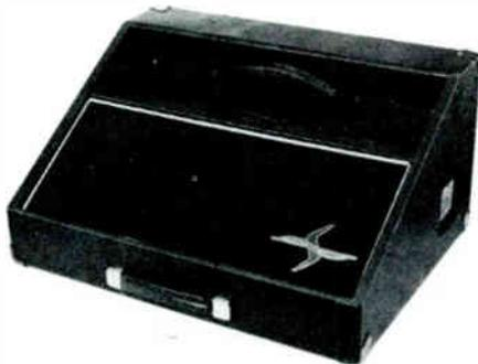
Professional, high-output, two-way monitor system designed on-stage use. Has two 8-inch speakers and a high-frequency driver coupled to a 120° radial horn. Horn dispersion angle may be reduced to 60° for tighter control of foldback signal. Can be positioned at 30° or 60° angle to the stage. Maximum recommended amplifier output: 100 watts continuous to 8 ohms, output 117 dB SPL at 1.2m (four feet) with 100 watts.
