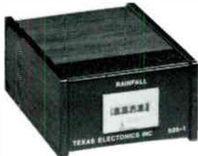
The 525-1 AC (which includes the Model 525 transmitter) is a single, 4-digit, counter console which contains a power supply for 120 volt AC operation. The 4-digit counter indicates up to 99.99 inches of rainfall and is reset to zero with a front panel-mounted mechanical lever.
