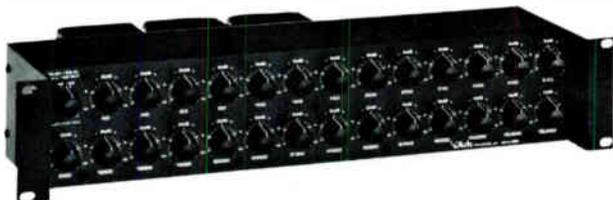
27 One-third octave bands from 40 Hz through 16 kHz. ±10 dB control range. 12 dB/octave high-pass filter variable from 20 Hz through 160 Hz. Noise better than -90 dBm. Accessory socket for optional low-level crossover networks. Barrier strip connectors.
