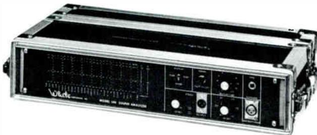
27 Double-tuned 1/3 octave filters on I.S.O. centers from 40 Hz through 16 kHz. 27 by 10 LED display plus separate dB-SPL and overrange readout. One and two dB scales. Display vernier. Built in pink noise generator. Mic and line level inputs. Sync and log amplifier outputs for remote oscilloscope display. Rugged road case. Metts ANSI S1.11-1971 Class II Specifications.
