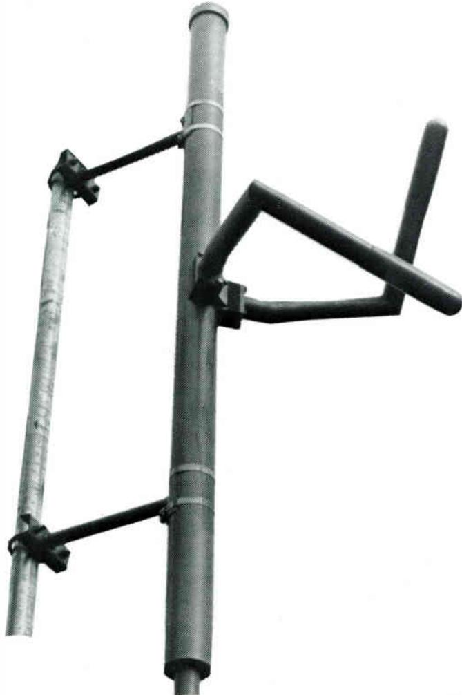
An extremely broadband low Q slot fed design with excellent circularity and axial ratio, no feed point straps, and large gap form factor.
