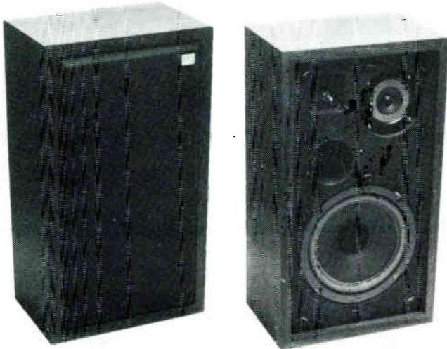
The MONITOR 2-way system incorporates an 8" woofer with a 14 oz. magnet in a ported cabinet; combined with an L-C cross-over network at 2800 Hz; L-pad, and a 1 3/4" phenolic ring tweeter with a 2.4 oz. magnet.
