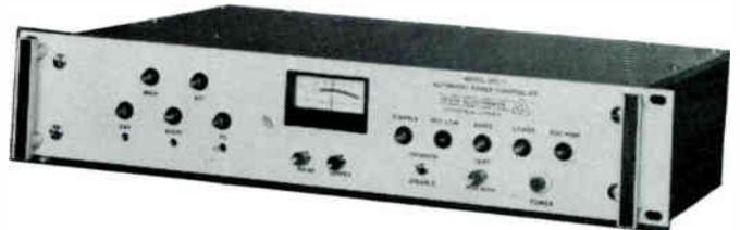
The APC-1 monitors the output power of either AM or FM broadcast stations; and by interconnection to the transmitter's Raise/Lower power controls, it causes the power to remain well within the F.C.C. limits. An optional ATS panel provides a means for incorporating the APC-1 into an ATS system.
