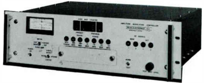
The AMC-1 utilizes a patented closed-loop concept to provide modulation enhancement. The AMC-1 detects and corrects over or under-modulation operation, as well as providing a digital display of the number of over-modulation bursts for the previous and present one-minute period. An optional ATS panel is available to make this product conform with the FCC requirements concerning modulation control in an automatic transmitter atmosphere.
