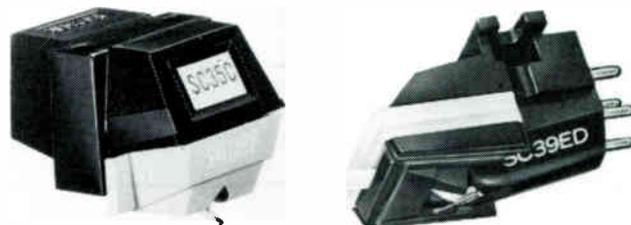
The SC35C is designed for use on the heaviest and most rugged tone arms which require a tracking force of 4 to 5 grams. The stylus assembly of the SC35C is rigid enough to withstand the punishment of continuous backcuing, yet compliant enough to offer excellent mid- and high-frequency reproduction.
