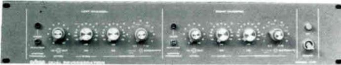
The integral "floating threshold limiter", exclusive to Orban/Parasound protects the spring against both overload and "boing" sounds. This circuit serves to eliminate sharp, sudden changes in level regardless of average level. This makes it possible to reverberate such instruments as guitar or drums for the first time with a spring system. The limiter makes sure that "twangs" are ducked out and masked by the direct sound mixed with the echo return.
