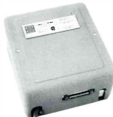
The ERC-19522 recorder coupler is used to connect customer provided recording equipment to a telephone line. The ERC-19522-22 recorder coupler is supplied with the ERC-19522-11 voice control unit factory-installed. The ERC-19522-21 or -22 recorder coupler may be used with individual or 2-party service. The ERC-19522-21 or -22 recorder coupler:
