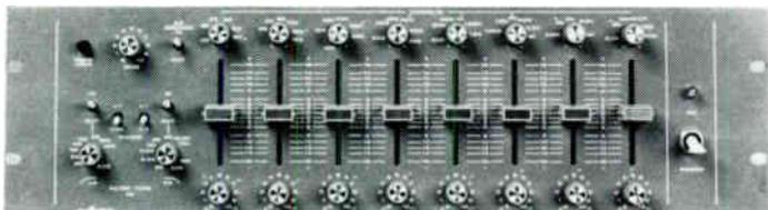
The ORBAN 672A is a cost-effective, professional, quasi-parametric equalizer with the convenience of graphic-type EQ controls. Wide-range high-and low-pass filters with 12dB/octave Butterworth slopes follow the graphic section for added versatility. The 672A has two outputs, arranged so that these filters can also be used as a full tunable electronic crossover.
