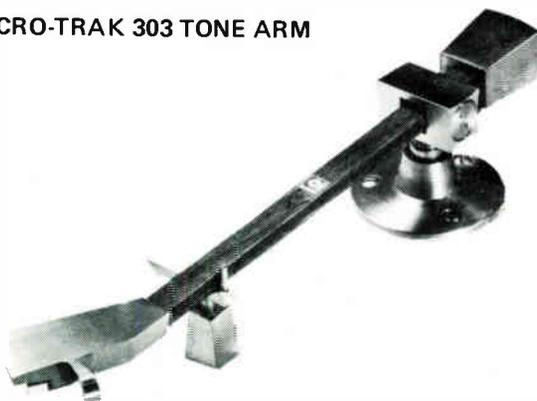
This tone arm features modern styling, plug-in memory balance head, laminated wood and epoxy body makes for rugged, light-weight construction. Stylus force once set is tamper proof, and adjusted by counter-weight. A standard of the industry.
