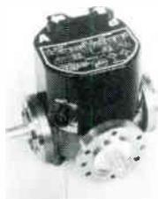
MCI Coaxial Transfer Switches are designed primarily for application in television, FM and AM broadcast transmitter plants, and HF, VHF, and UHF communications systems. As four-port transfer switches they will switch two signal sources between two loads. Since they can also be used as SPDT switches, complex switching matrices can be easily assembled.
