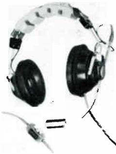
Professional, binaural headphone and wide range, omnidirectional, dynamic boom microphone for live, remote broadcasting. Non-metallic headphone and microphone elements resist environmental extremes for precise transmission and reception under all conditions. Supplied with 2 meter un-terminated cord and in-line "push-to-cough" switch. Padded headband and ear cushions. Black with grey trim.
