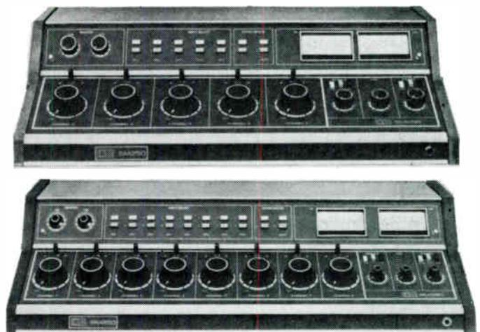
Featuring ladder-type maintainable step attenuators with cue bus switching, telephone-type channel keys and contact-free FET bus selection. Separate monitor, headphone and cue channels. Field proven 3600 Series modular plug-in electronics. Two input pushbutton pre-selection and microphone or high level capability (cont.)
