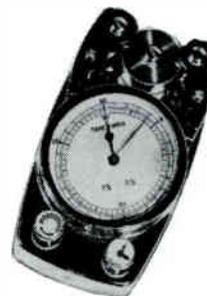
Precise tape or speed measuring device with scale calibrated in minutes and seconds at 7.5 and 3.75 ips. Features time reset knob and strobe disc for speed checks. Use with reel-to-reel decks, cart machines and tape winder.
