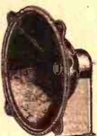
The new Model D-9 is designed for operation with all types of amplifier systems and particularly for latest model receivers. Ideal for new set builders and for replacement purposes. In the 12 inch cone class, and equipped with mounting support and 30 inch cords. All models have 2,500 ohm field coil.
