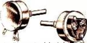
A well-known, attractively-priced selection of dependable high-quality volume controls. Insulated shaft type. C—Clockwise Taper; CC—Counter Clockwise Taper. All others with uniform taper. 1 1/2 inch shafts may easily be cut to shorter length. 3/16" bushing. May be had with or without AC line switch.
