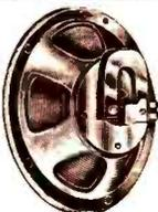
A sturdy and powerful, small size magnetic speaker, only 8" in diameter. Has heavy pressed steel frame and large magnet. Latest improved armature design; extra flexible diaphragm. Will handle up to 1 watt output. DC resistance, 1000 ohms. Especially recommended for battery and AC-DC set use, as an extension speaker, or in multiple-speaker installations. An ideal high quality all-purpose unit constantly in demand and priced low for profitable installations. Shipping weight, 4 lbs.
