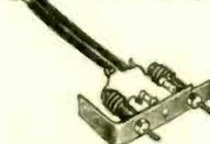
Eliminate TV interference and images from adjacent channels. For channel FM broadcasting stations and signals from 14 to 28 mc Amateur stations. Have ceramic condensers and powdered iron-core slug-tuned coils to eliminate interfering frequencies. 5" twin line connecting ribbon with tinned lugs. Bracket, 2 1/4 x 1 1/2". With instructions. Shpg. wt., 4 oz.
