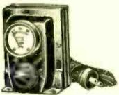
Type T10306. 150 VA constant duty, manually operated variable transformer. Adjusted by turning rotary tap switch. May be used as step-up or step-down transformer to correct either low or high voltage line condition. Calibrated voltmeter accurately indicates secondary
