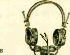
Fig. A. Brandes "Supiorior" Phones. A high quality, ruggedly-built headset which has been a favorite for years. Outside terminal type, with metal cases and bakelite caps. Diaphragm diameter is 2 1/2". Has double coils, two in each receiver. Flexible metal split headband is easily adjustable for maximum comfort. Supplied complete with 4 1/2-foot cotton-covered cord. Magnets of high retentivity are 1/2" square. Resistance, 2000 ohms per pair. Shpg. wt., 13 oz.
