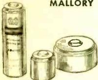
Features extremely long shelf life and uniform discharge voltage. Unique design permits indefinite storage. Voltage approximately 1.345 v. through entire life. Unaffected by temperatures as high as 250° F. or pressure ranging from a high vacuum to thousands of pounds per square inch. Resistant to humidity. Ideal for use as a secondary voltage standard.
