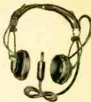
Power rating, 75 milliwatts. Impedance, 8 ohms; may be matched to either 600 ohm or 50,000 ohm sources with plug-in transformers listed below. Rugged five-foot cord constructed of rubber-covered cadmium-bronze wire for long life, high flexibility. Cord is terminated in a two-circuit plug for convenience in connecting to a tuner or communications receiver. Shpg. wt., 12 oz.
