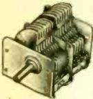
Fig. B. J. W. Miller 365 Mmf Condensers. Compact TRF variables. Have trimmers on side of frame. Outer rotor plates are slotted for tracking adjustment. Tapped holes in frame provide secure mounting. Range: 10 to 365 mmf. Shaft diameter,  $\frac{3}{8}$ ". Type 2112:  $2\frac{1}{2} \times 1\frac{1}{2} \times 1\frac{3}{8}$ ". Type 2113:  $3\frac{1}{2} \times 1\frac{1}{2} \times 1\frac{3}{8}$ ". Shpg. wt., each, 6 oz. 60 H 725. Type 2112. 2-gang. NET.....2.06
