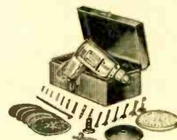
Drill kit with extra-power, 3/8" geared-chuck drill. Drill has speed of 610 rpm under load—permits accurate control for drilling steel, masonry, concrete, etc. Provides ample power for screwdriver attachment, wood boring to 1 1/4", hole sawing to 2". Includes: 5—5" sanding discs; 5 1/2" wool polishing bonnet; 5" rubber backing pad; steel paint mixer; set of 6 wood augers (3/8" to 1"); 9 drill bits. In steel case, 12 x 7 1/4 x 5". For 110-120 v., 60 cycle AC. Wt., 10 lbs. \$2.00 Down.
