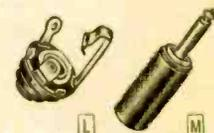
Standard  $\frac{1}{4}$ " 2-conductor phone plug and jack. Plugs have screw-type terminals and are available with either red or black bakelite handle; all metal parts, except screws, have nickel plating; overall length, 2 $\frac{1}{2}$ ". Open-circuit jack has  $\frac{3}{8}$ " dia. threaded shank  $\frac{3}{8}$ " long; requires 1" behind panel. Av. shgp. wt., 3 oz.
