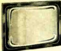
Solid, optically clear, ½" thick plastic safety masks for rectangular picture tubes. Prevents tube breakage and guards against "implosion" and "shattering". Gold metal luster finish border. Easy to install. Shpg. wt., 1½ lbs.
