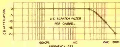
Found only in the finest high-fidelity equipment, a pair of genuine L-C type scratch filters (with a choke for sharp cut-off), are used in the Knight-Kit Stereo Preamp Kit to eliminate scratch without affecting mid-range frequencies.
