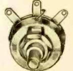
Precision units developed especially as controls in drive-in theater speaker installations. Withstand extremes of temperature and humidity. TSA-10 is an L-pad with 10-ohm input and 4-ohm output. TSA-35 is a 35-ohm series-type potentiometer. TSA-6 is a 6-ohm shunt-type attenuator. 1 1/2" dia. cases. Shafts are 1/2" long; steel knurled. Brass. Shgp. wt., 4 oz.
