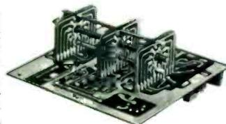
**Two Printed Circuit Boards.** Virtually all circuitry (RF, oscillator, converter, voltage regulator, IF, audio, BFO and rectifier stages) is on two printed circuit boards. Greatly simplifies construction, and makes an extremely important contribution to stability and overall performance.
