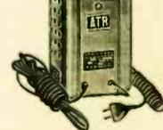
Model 612CA6. Charges 6 or 12-volt storage batteries through cigarette lighter receptacle of any vehicle. 6 amp charge rate tapers to 3 amp. Circuit-breaker eliminates need for fuses. For use in negative and positive-ground vehicles. 8 1/2 x 5 1/2 x 3 3/4". For 110-120 v., 50-60 cycle AC. Shpg. wt., 8 lbs.
