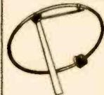
**Model HH-6 Halo.** Mobile antenna for 6 meters. Offers high mechanical stability and minimum wind resistance. 1" dia. tubing. Weather-sealed. Matches 52 and 72-ohm coax. Fits any standard mobile mount. Less mast. Wt., 5 lbs. 77 CU 868. NET **12.95**
