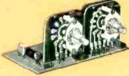
The use of printed circuit boards, exclusive printed circuit switches, and PAC units (complete resistor-and-capacitor plug-in assemblies) simplify assembly—you'll marvel at the ease with which you build this deluxe unit.
