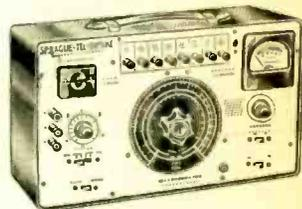
Multi-purpose bridge-type capacitor analyzer for radio-TV servicemen. Valuable time-saving aid—quickly detects open, shorted, or intermittent capacitors. Provides an accurate, multi-range capacitance and power factor measuring bridge; an insulation resistance checker for paper, mica, and ceramic capacitors; a leakage current indicator for electrolytics (tests at rated voltages); and a turns ratio scale to measure turns ratio of power and audio transformers.
