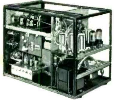
**Girder Construction.** Steel cabinet on girder frame for exceptional strength and rigidity.
