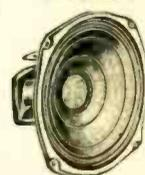
Jensen's highly popular "Concert Series" PM speakers. DP-Alnico V magnets for exceptionally high efficiency and distinct reproduction. Cones are selected for maximum frequency response characteristics. Rigid frame maintains proper alignment of voice coil and magnet structure. All speakers listed below have 3.2-ohm voice coil impedance, except Type P275-Y which is 16 ohms (for transistor radios). All except P275-Y and P4-W have bracket for mounting matching transformer.
