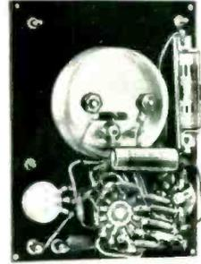
Film-type precision multiplier resistors provide high accuracy and continued dependability.
