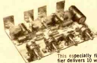
This especially fine transistor stereo amplifier delivers 10 watts per channel continuous power (RMS) into any 8 ohm speaker. The
