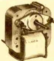
Rugged, GI open frame shaded pole motor for continuous operation such as blowers, pumps, fans, animation, gear trains and many other hobbyist applications. 3500 RPM C/W rotation. Has oil-less type bearings. Shaft 3/16" dia. x 1 1/4" long. Body 2 3/4" wide x 3" high x 2" deep. Shpg. wt., 2 lbs.
