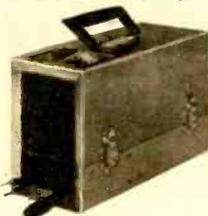
Hundreds of uses: Operates TV's, power tools, barbecue motors, lights, hedge clippers, or, appliances using 117V., 60 cycles AC. Has self-contained 25 amp, rechargeable wet storage battery. Frequency stable within ½ cycle with load changes. Plugs into AC outlet, or, car cigarette lighter to recharge battery. Has automatic overcharge protection. Meter shows charge rate and hours of anticipated output. Size: 12x5½x8". Shpg. wt., 36 lbs.
