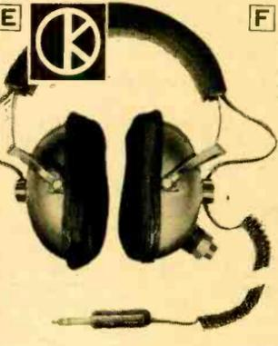
Fluid-filled cushions seal out noise. Dynamic transducers. Shatterproof construction. 20-20,000 cps. 4-16 ohms. 10' retractable cord. Shpg. wt. 2 lbs.
