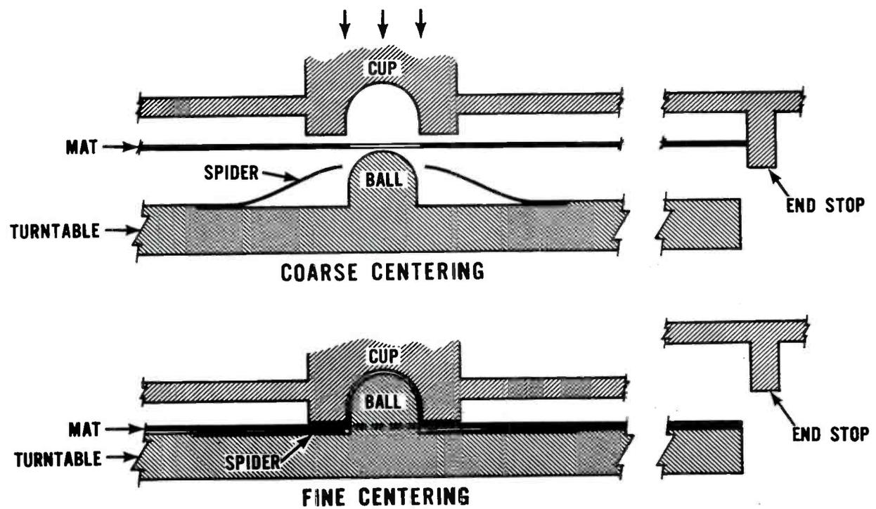
Fig. 4 POSITIONING OF THE MAT
