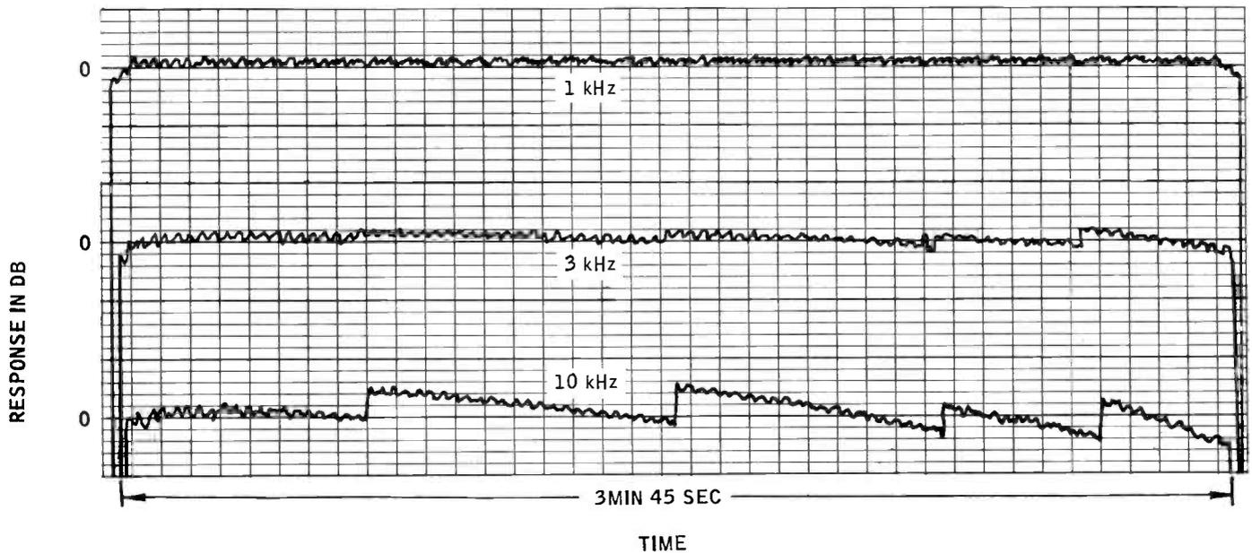
Fig. 10 1 kHz, 3 kHz, and 10 kHz RESPONSE VERSUS TIME
