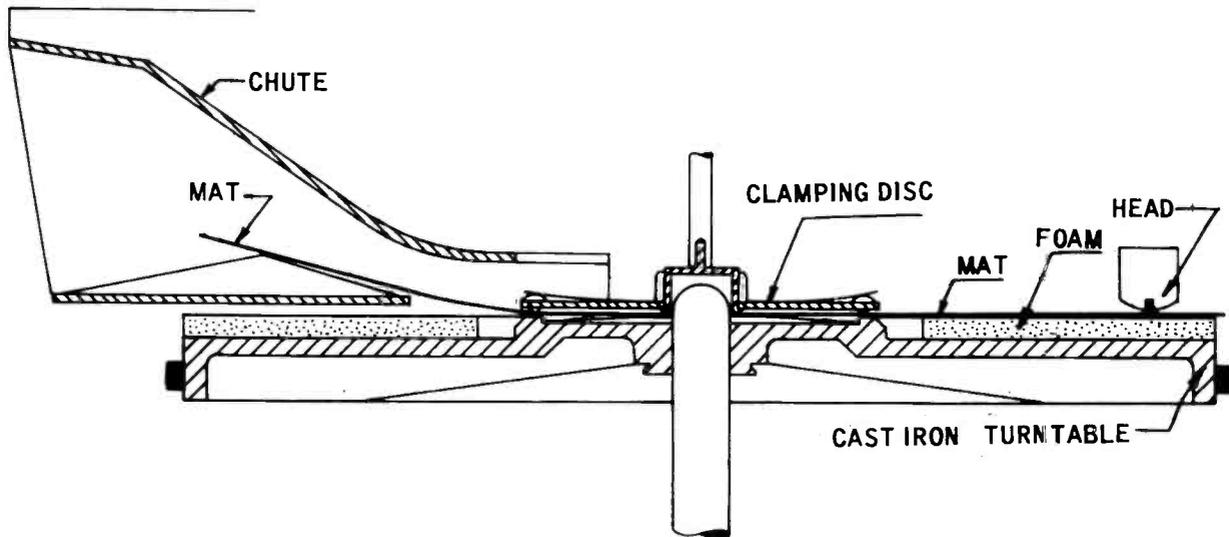
Fig. 5 SECTIONAL VIEW SHOWING POSITION OF MAT AND HEAD IN PLAY MODE
