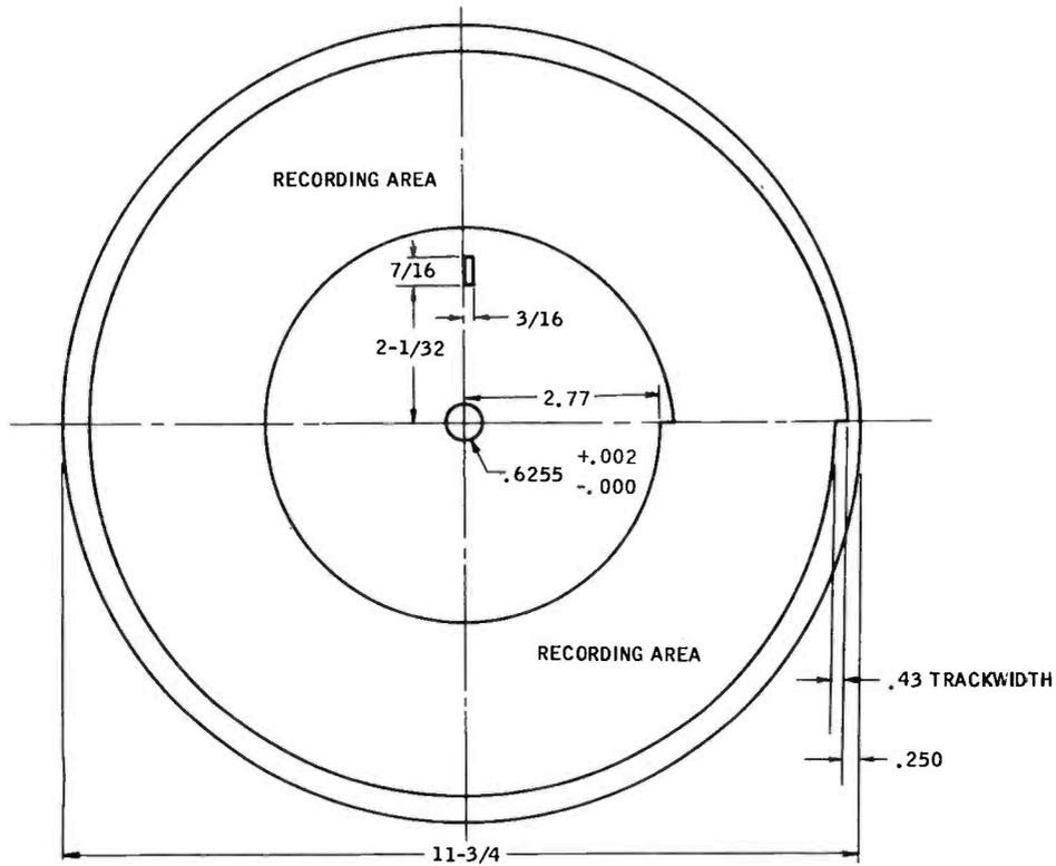
Fig. 1 AMPEX CUE MAT - THICKNESS 3 MILS
