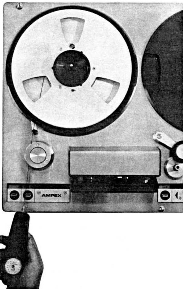
Fig. 4-2. *Checking Holdback Tension*
