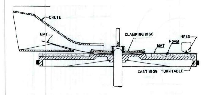
Fig. 5 SECTIONAL VIEW SHOWING POSITION OF MAT AND HEAD IN PLAY MODE
