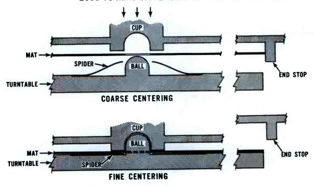
Fig. 4 POSITIONING OF THE MAT
