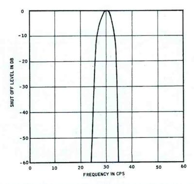
Fig. 12 PILOT TONE SHUT OFF SENSITIVITY VERSUS FREQUENCY
