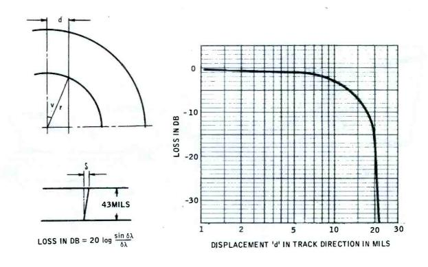
Fig. 3 GEOMETRY OF HEAD MOTION AND IO-KC INSIDE TRACK LOSS VS HEAD DISPLACEMENT IN TRACK DIRECTION
