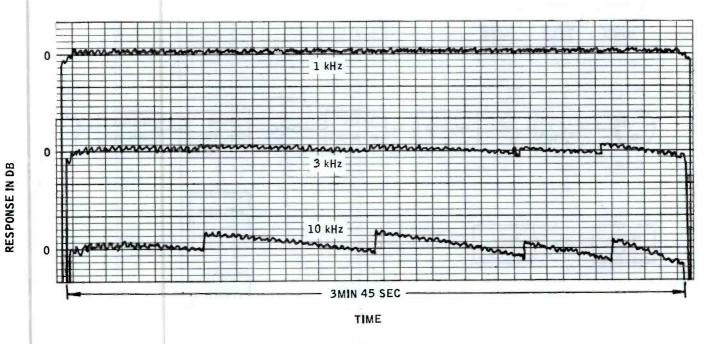
Fig. 10 1 kHz, 3 kHz, and 10 kHz RESPONSE VERSUS TIME
