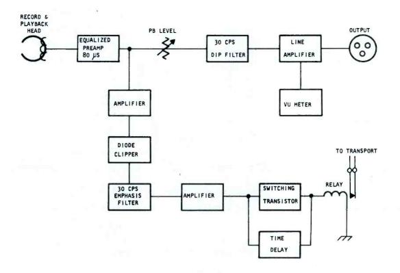
Fig. II REPRODUCE CIRCUIT BLOCK DIAGRAM
