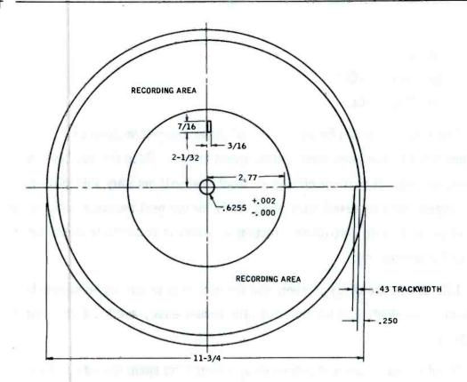
Fig. I AMPEX CUE MAT - THICKNESS 3 MILS
