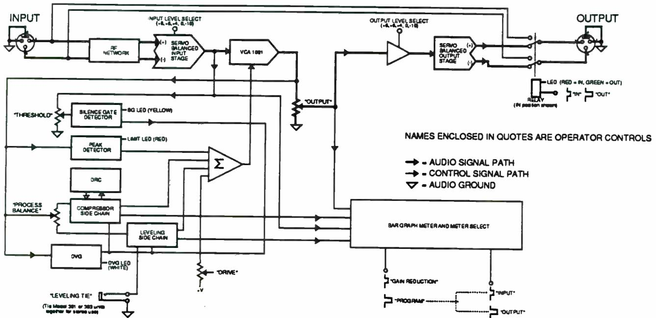
Fig. 2-2. Block diagram of COMPELLOR Model 301 circuits.
