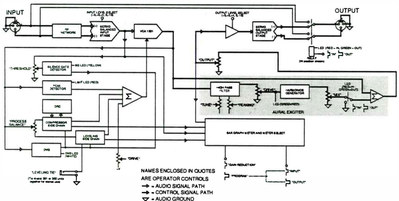
Fig. 2-3. Block diagram of COMPELLOR Model 303 circuits.
