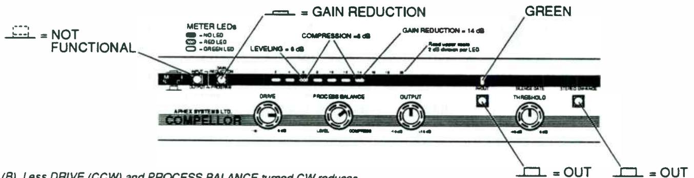
(B) Less DRIVE (CCW) and PROCESS BALANCE turned CW reduces GAIN REDUCTION but increases Compression.
