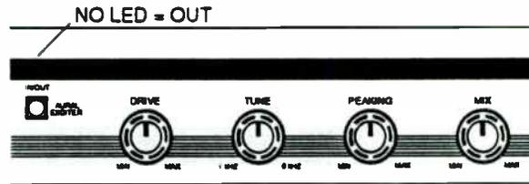
3. Slowly increase the MIX Control (CW), until you begin to hear the extra edges and minute cues missing from the original signal. (See OPERATIONAL CHARACTERISTICS of AURAL EXCITER, Section 2.1.7)
