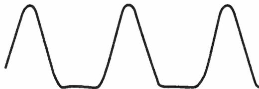
Fig. 7-3. Waveform shape appearing at clockwise terminal of MIX pot.
