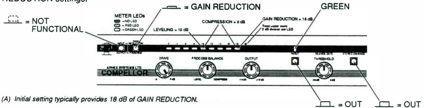
(A) Initial setting typically provides 18 dB of GAIN REDUCTION.
