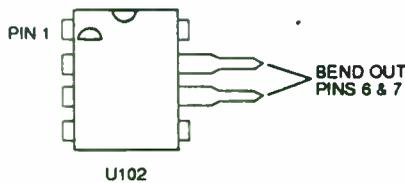
*Fig. 8-6. An illustration showing what pins 6 & 7 should look like once the modification has been completed.*
