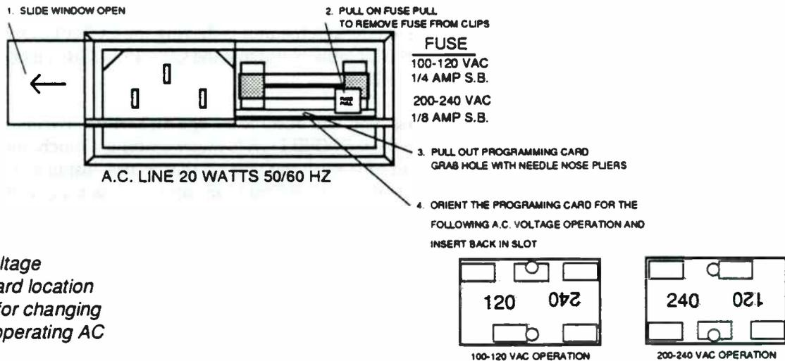
Fig. 3-4. AC voltage programming card location and procedure for changing COMPELLOR operating AC voltage.
