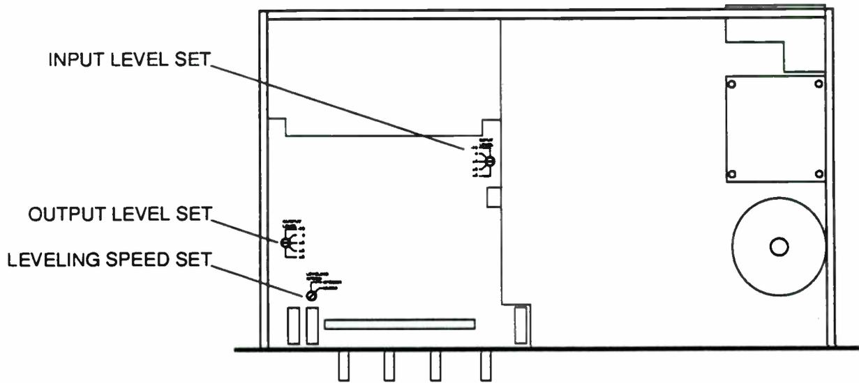
*Fig. 3-1. Simplified top view showing location of INPUT LEVEL SET, OUTPUT LEVEL SET, and LEVELING SPEED SET on the Audio Processing Board, common to both COMPELLOR Model 301 and 303 units.*
