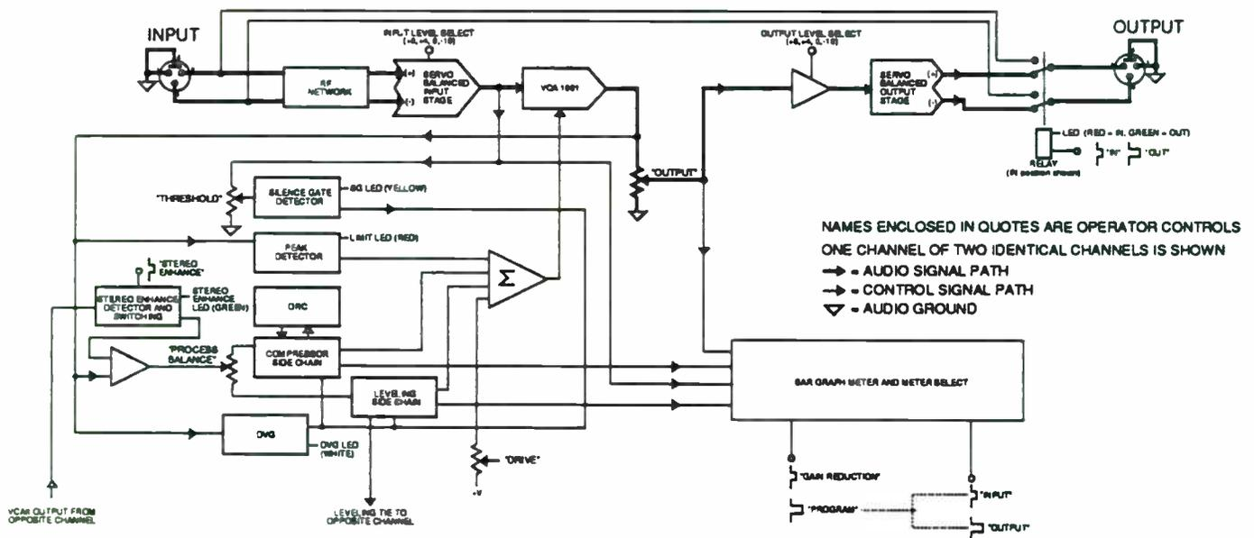
Fig. 2-1. Block Diagram of COMPELLOR Model 300 circuits. Only one channel is shown.
