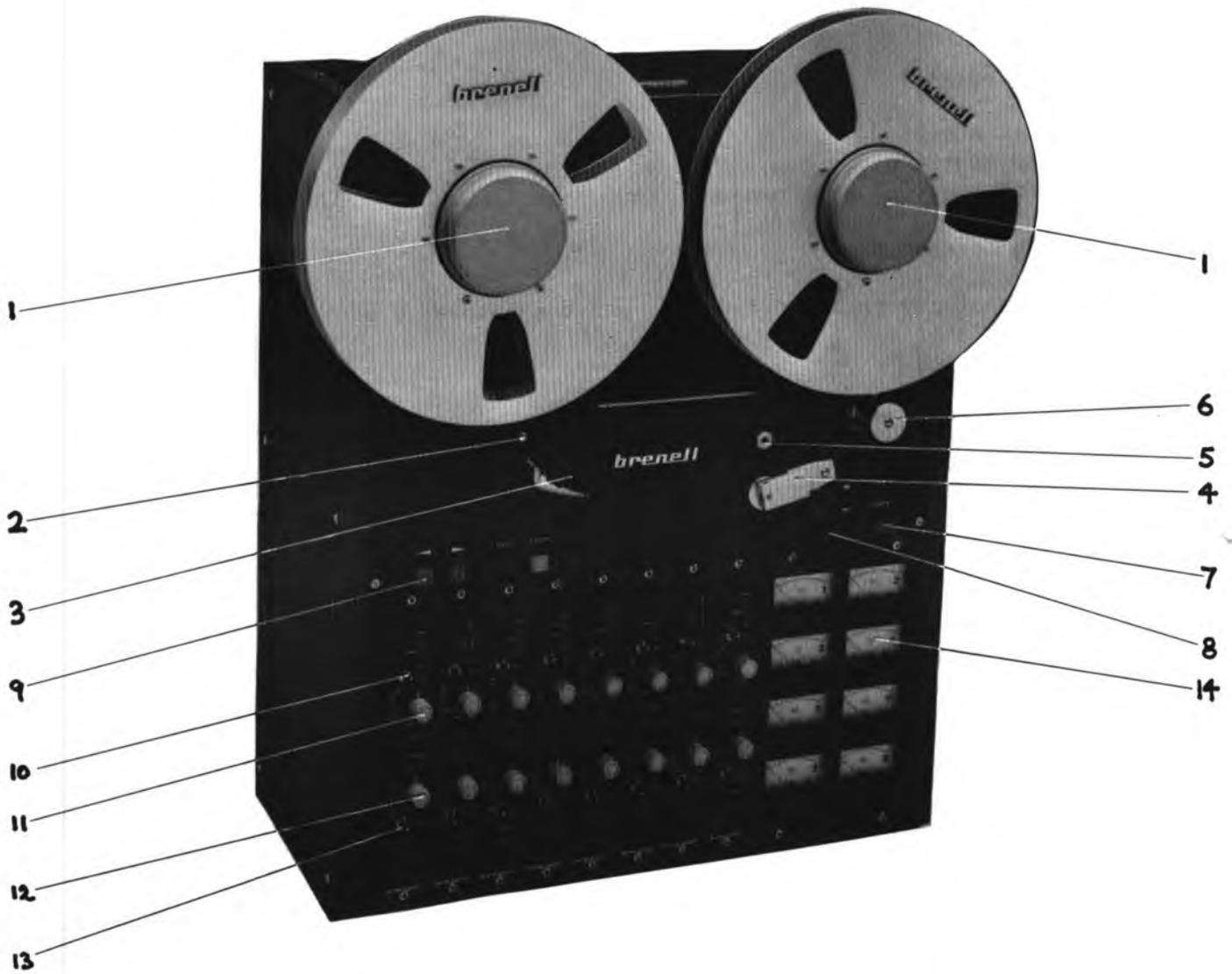
When the deck is in the record mode the red indicator adjacent to the mode selector pushbuttons will light.
