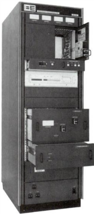
Front view of FM-1.5A Transmitter illustrates modular slide out construction.
