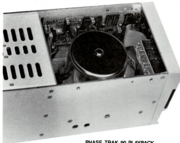
PHASE TRAK 90 PLAYBACK DC Servo Motor Assembly
