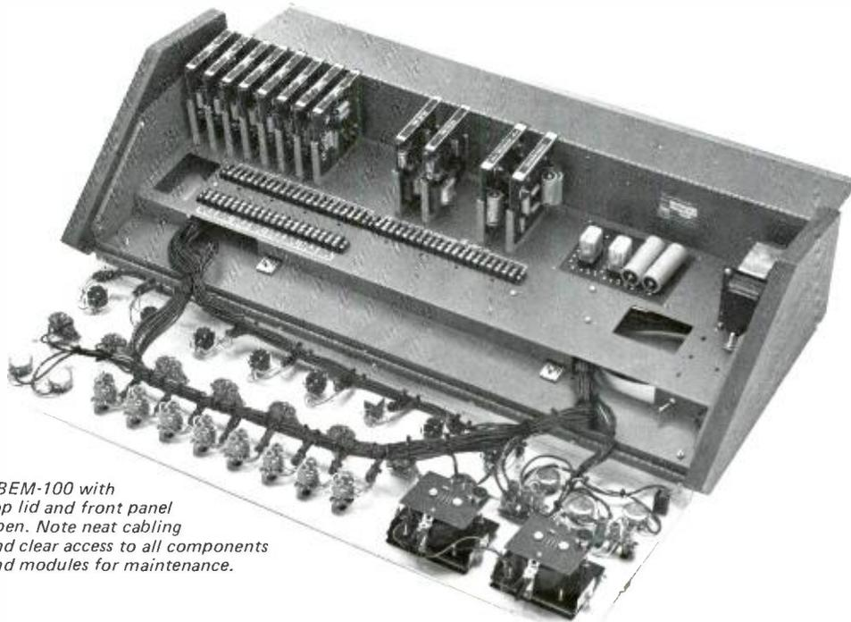
*8BEM-100 with top lid and front panel open. Note neat cabling and clear access to all components and modules for maintenance.*
