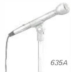
**635A:** Smooth, carefully chaped response yields "flat effect" when used close up. Built-in four-stage pop and breath blast filter. Cable and mounting clamp furnished. Response: 80 to 13,000 Hz. Lo-Z. Output level: -55 dB.
