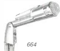
**664:** Designed for quality tape recording, communications, and public address applications. Cardioid at all frequencies. Response: 60 to 15,000 Hz. Output: -58 dB. Stud mount with on/off switch. Cable furnished. Satin chrome.
