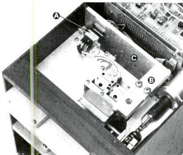
The 5300A front panel is hinged, the decks pull out, and all electrical connections to the deck are made through a single plug in connector **A**.
