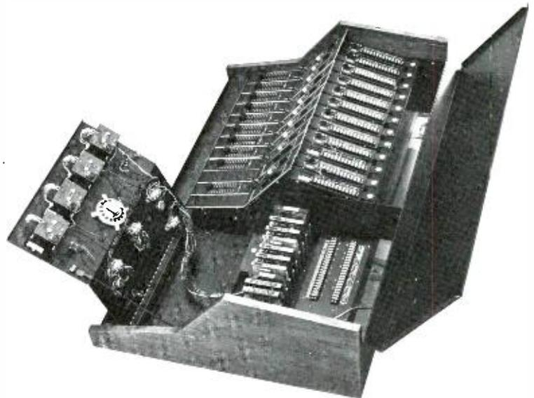
*Model SL-4100 with top and right-hand front panels open. Input cabling readily terminated on input module top barrier strips. Output barrier strips at lower right. System plug-in electronic modules and secondary front panel controls and switches readily accessible. Installation eliminates all exposed cabling.*
