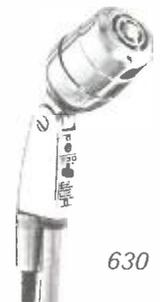
**630:** Famous for quality at low cost. Unaffected by heat or humidity. Dual Lo-Z or Hi-Z. E-V QC -4M cable connector allows easy change of impedance by moving a single pin. Response: 60 to 11,000 Hz. Output: -55 dB. On/Off Switch. Satin chrome finish. Cable furnished.
