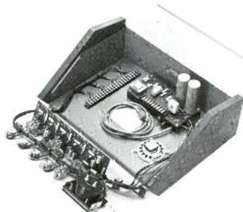
*Hinged top cover and front panel give full access to the barrier strips for installation and all control switches and components for maintenance.*
