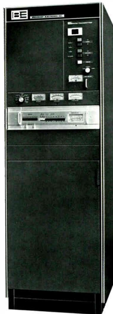
**BROADBAND, SOLID-STATE IPA** — A single broadband module using one (1) Type CD-4262 balanced RF power transistor serves as the IPA in the FM-3.5 transmitter. This driver module is conservatively operated at about 50% of its maximum rating, so there is plenty of reserve power in the IPA stage.
