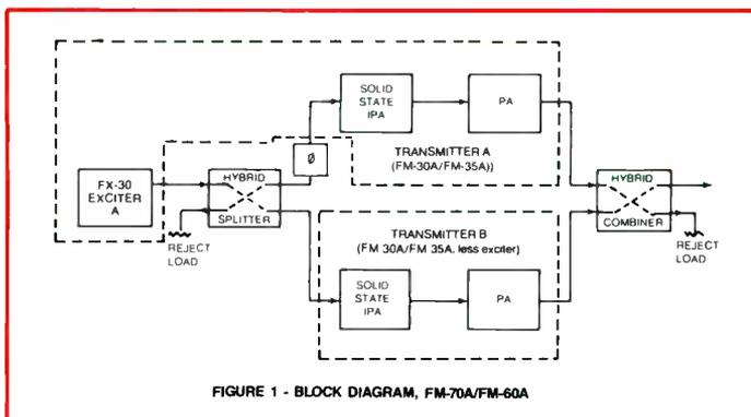
FIGURE 1 - BLOCK DIAGRAM, FM-70A/FM-60A
