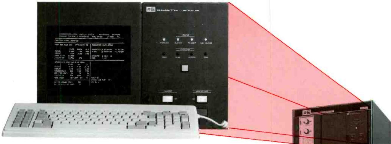
Five plug-in cards for the optional microprocessor system are housed behind hinged Transmitter Controller panel. To left is CRT monitor for bar-graph and tabular information read out display, and keyboard for message programming and display page access.
