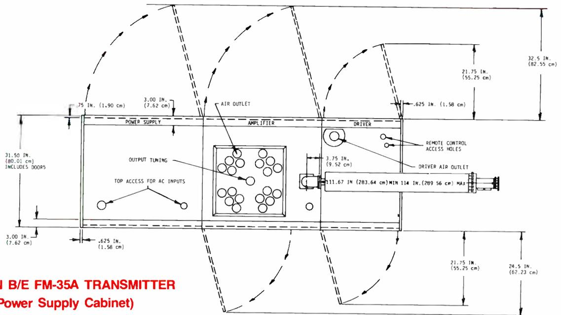
**FLOOR PLAN B/E FM-35A TRANSMITTER
