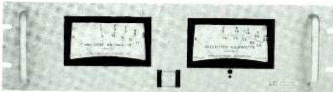
Installations which do not require the fast response time and the forward-power drop-off alarm of model 3171 are protected from high VSWR by WATTCHER MODELS 3127/3128.
