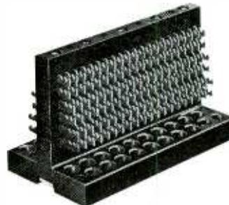
The ADC 20-Pin Terminal Blocks are molded of durable, black, thermoset plastic per Military specifications MIL-F-14F. Terminals are brass with a tin allow plating for lasting solderability. The PJ-101 series blocks have terminals graduated in length for ease of wiring. All Terminal Blocks are numbered along the top row for easy terminal identification.
