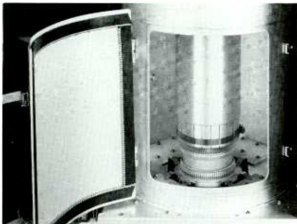
Computer optimized coaxial cavity employs BE's patented folded half wave tank circuit which eliminates the plate blocking capacitor and all sliding contacts in the output circuit.
