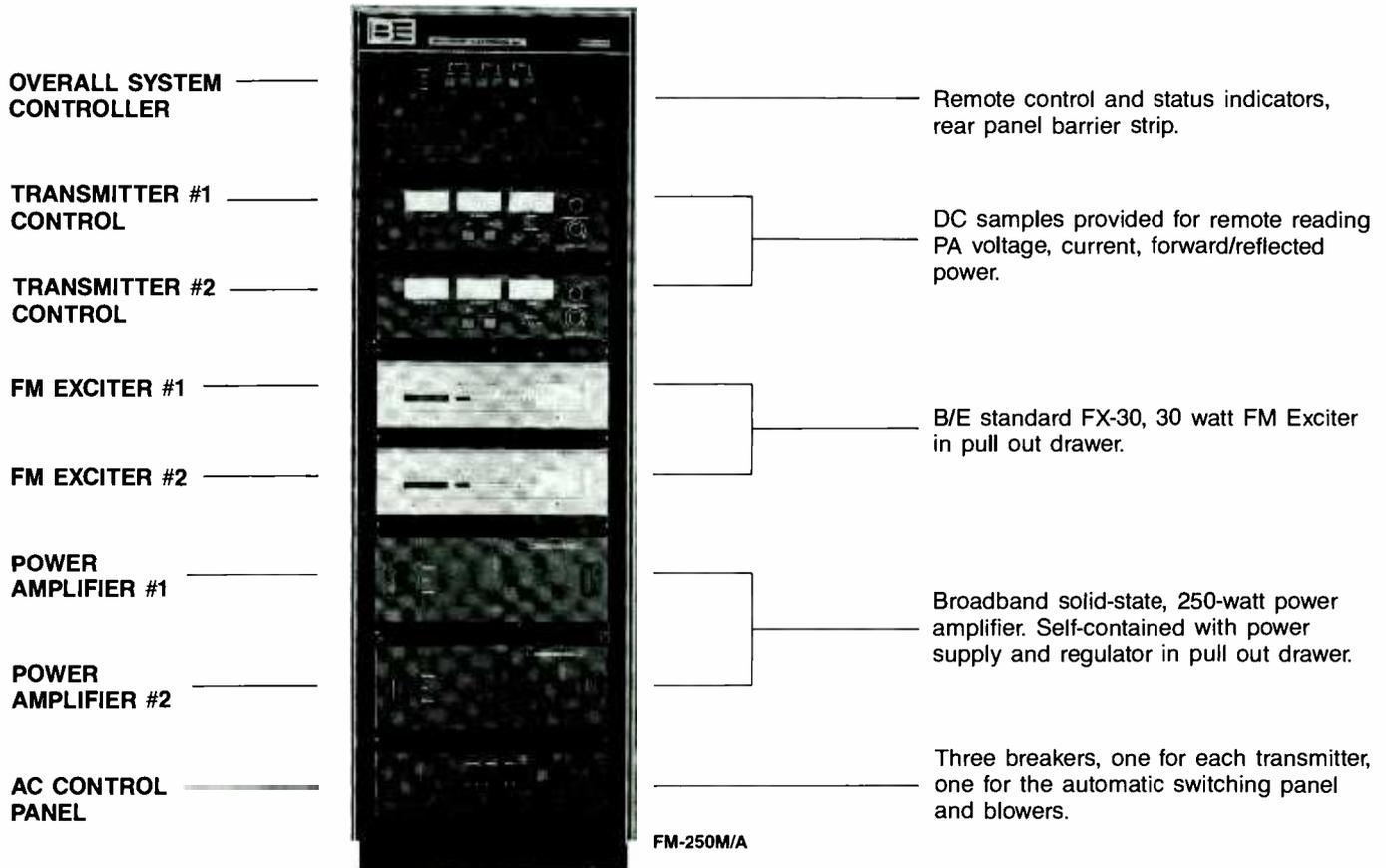
Broadcast Electronics' Model FM-250M/A transmitter system is composed of two 250 watt solid state FM transmitters designed to a fully redundant main/alternate main configuration for continuous operation on one specified frequency in the 87.5 MHz to 108 MHz FM broadcast band.
