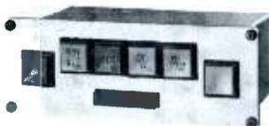
Remote control available for complete external control of all functions. Suitable for mounting in console desk cut-out or in blank rack panel. Measures 2.25" high x 4" deep x 5.5" wide. Mating 24-pin connector furnished and we will fabricate pre-wired cabling to length.
