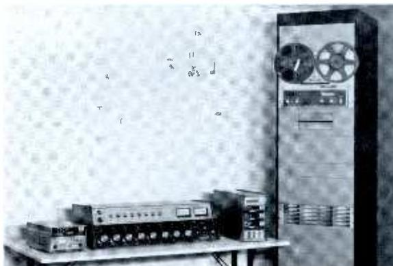
The need for a delay device in broadcasting, especially for talk shows, has been obvious for many years. Spotmaster produces many delay devices from single deck machines to more complex systems such as the one shown here. These systems are practical enough to be operated by a single person with ease and complete safety.
