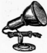
**WEATHER-PROOF** Cadmium plated **OUTLET-BOX** type bracket for ANY Reflector, Projector, or Heat lamp. Adjustable to direct beam of light in ANY direction. May be fastened direct to 4" outlet box, or by screws to any surface. All steel; bakelite socket. Base 1 1/4" dia. Wt. 1 1/2 lbs.
