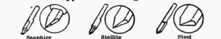
**Sapphires**—Hardest point with lowest friction make the finest cutting points and are the longest wearing. Can be resharpened.
