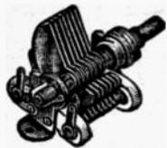
Cadmium-plated soldered brass plates; Isolantite insulation; heavy aluminum ends; single-hole mount; .0245" gap; .0225" plates; 1/4" shaft, can be ganged; silver plated Beryllium wiper; 500-volt a.c. test.
