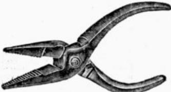
Weighs only 1½ ozs., a handy pocket pliers—and because it's shock-proof and non-magnetic—it can be used on apparatus while in operation. 6000-V. breakdown, heat resistance 240 to 300°. Tensile strength of material, 6,000 lbs. per sq. in.
