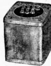
Filament Transformer. Primary input 110 Volts 60 cycle. Secondary 5 Volt C.T. at 10 amps or primary input 220-240 Volts, secondary 10 Volts C.T. at 10 amps, 2000 Volt insulation with heavy duty solder terminals. Fully encased in grey enameled heavy metal case 4"x3½"x5" with mounting holes tapped for standard screws.
