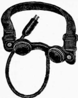
To be worn around neck. Consist of two carbon mike buttons in molded rubber throat pieces. Designed especially to pick up speech and exclude outside noise. Can be used with any low gain amplifier. Requires 50 to 100 ohm mike transformer and any 4½-volt battery. Current drain 100 ma. Has many possibilities for PA, Amateur and Experimental applications.
