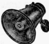
Model 1B8 Complete Directional Speaker; 60° dispersion; frequency 300-5000 cycles; 13-WATTS, 8-ohm voice coil. Projects to 1/5 mile. Hermetically sealed BUILT-IN DRIVER UNIT. Complete with mounting bracket, height 9", dia. 9"; wt. 5 lbs.
