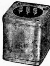
Filament Transformer. Primary input 200, 220 or 240 Volts, 60 cycles. Secondaries 5 Volts at 3 amps, 2.5 Volts at 10 amps. Secondary terminals on insulated bushings for high Voltage uses. Fully encased in grey enameled heavy metal case 3½"x3½"x4½" with mounting holes tapped for standard machine screws.
