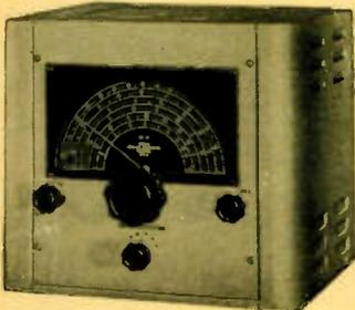
For added sensitivity, image rejection and gain when used with any communications receiver. Range 550 KC to 33MC. Built-in power supply. Tubes are 2-6K7 and 1-80. Cabinet matches current RME receivers in every detail. Operates on 115 V. 60 cycle AC.
