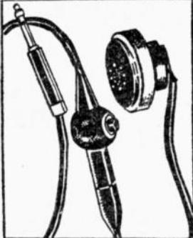
Single Button Carbon Mike. Has press to talk switch in rubber-covered flexible cord 4 1/2 ft. long, complete with standard 3-circuit plug. Has separable plug-in cord between switch and mike. Can be used with any low gain amplifier. Requires 50 to 100 ohm mike transformer and any 4 1/2 V. battery. Current drain 100 MA. Ideal for mobile transmitters, also has many possibilities for PA, Amateur and Experimental applications.
