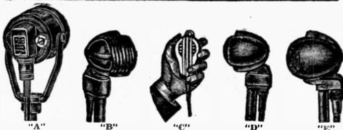
**"A":—MODEL U-9S VARIABLE IMPEDANCE DYNAMIC — ONE MICROPHONE FOR ALL NEEDS; impedances of 50-200-500 OHMS or HIGH IMPEDANCE available by the twist of a switch on the back! ADJUSTABLE for semi or non-directional use, Model U-9S is completely free from peaks and holes over its frequency range of 40-9,000 cycles. Output level at high impedance is minus 59db. Professional in construction and appearance, tilting head, complete with 20 ft. detachable cable; gun metal finish.**
