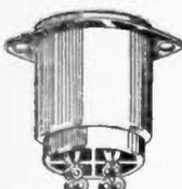
For 2x2 rect. and other tubes with base diameter of 1.156". Widely used in TV. and Photo Flash equip. Socket set at bottom of a deep molded bakelite shell. Steel mtg. plate molded into shell. Mtg. holes on 1 7/8" centers. Mounts from above or below in 1 1/2" hole. List Price, \$1.50.
