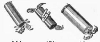
(A) and (B) are popular cardboard tubulars with inner seal and ample wax seal at ends and flexible insulated leads. The single units (A) are provided with feet for vertical mounting in addition to an adjustable strap with each for horizontal mounting like on Dual unit (B). Type (C) are encased in aluminum cans with threaded necks for mounting.
