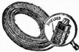
Needed for many applications. Size 20, stranded tinned conductor with vinylite insulation, cotton braid and overall tinned copper shield. Single Conductor.
