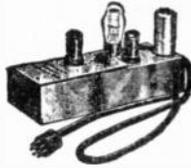
An extremely stable variable frequency exciter with band switching, accomplished by a 6-position shielded coil turret. A front panel crystal socket has 1/2" or 3/4" pin spacing. Power output is in
