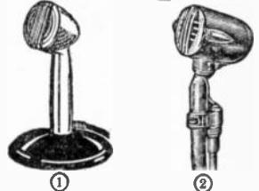
① **MODEL 200 CRYSTAL "VELVET VOICE".** A general purpose microphone and stand with detachable base to use for recording, PA, etc. Beautiful rich gold finish with chrome grille. High impedance, smooth frequency response 30/10,000 cps. —50 db. Threaded for 5/8"/27 stand. Overall height, 8". 15-ft. shielded cord attached.
