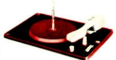
Center action type changer has a 3 second change cycle. Records are dropped by positive acting record release in spindle. **Single Tone Arm** is properly balanced for playing both 33 1/3 and 45 RPM records—May be moved at any time during play without damaging mechanism. Plastic snap inserts are used in large center hole of 45 RPM records.
