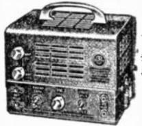
① 125-watt C.W. Kit with band switching exciter covering 3.5-30 MC in six bands completely self contained, features ease of construction, panel selection of six crystal frequencies, separate 350 and 1000 volt power supplies, exciter keying, meter switching and adj. link output coil.
