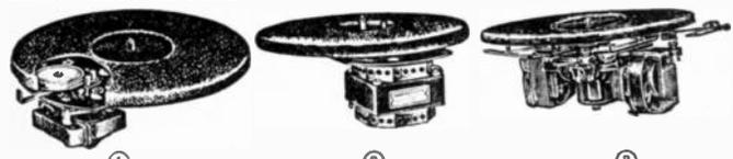
① New "G.I." Model "TS" Three-Speed Phono Motor. 33 1/3, 45, 78 RPM for playing any brand of records. 78 RPM direct from motor shaft; Neoprene belt drive for 33 1/3 and 45 RPM. Simple speed indicator lever changes speeds instantly on 8" turntable. Affords top reproduction of the new 33 1/3 and 45 RPM records with minimum of "wow" and rumble. Mounting plate 3 1/8 x 2 1/4", extends 2 9/16" below. Weight, 4 lbs. **\$6.51**
