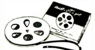
Paper base tape designed for unmatched performance in any magnetic tape recorder. Has high fidelity with freedom from background noise and distortion. Precision developed and made. 1250 ft. of tape on standard 7" aluminum reel gives 33 minutes of recording, time at 7 1/2" per second speed and 1 hours time at 3.75 inches per second.
