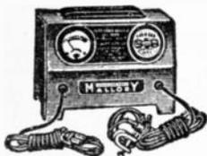
With trouble-free dry disc rectifiers and auto type fuse to protect the charger from improper connection to battery, and from serious overloads. Charges at maximum rate at start, decreasing as battery becomes fully charged. May also be used for electroplating, toy and model train operation, loud speaker fields, coin machines, and other applications requiring low voltage D.C.
