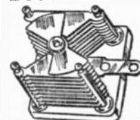
A new butterfly type condenser for use in balanced VHF circuits requiring a great amount of electrical and mechanical stability. All soldered sealed ceramic end plate 3/8" single hole mounting and 1/4" diameter x 7/16" slotted shaft. Rotation from min. to max. capacity 90°. Air gap .030". 1200-volt test. Capacity ratings are for each section. Size, 1 3/8" square, 1" to 1 1/2" deep.
