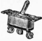
CH Type AN-3022-1B. Rated at 35 amps at 24-volt and 5 amps at 125-volt. Mounting centers 1 13/16" on mounting plate 3/4 x 2 1/16".
