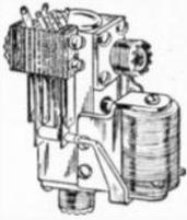
For use with 52 or 75 ohm RG Coax Cable. Has 1/4" pure silver SPDT internal contacts supported directly from cable connectors. Housing is aluminum, with end inspection port. Connectors are standard Amphenol 83-R. Max. rating 880 watts at 100 MC. Operates on 110 V. 60 cy. A.C. Size 1 3/8 x 2 7/8 x 3 1/2".
