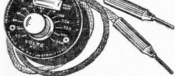
Just rotate the knob until glow lamp goes out and read voltage direct from the calibrated scale. A handy, portable instrument that can stand knocking around. Resistance approx. 1/2 megohm. Neon indicator good for 10,000 hours actual operation. Has flexible leads and test prods. Bakelite case dia. 2".
