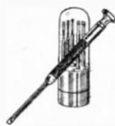
Blade sizes: .100", .080", .070", .055", .040". Handle length 2 3/4"; overall length 4 1/8". Blades are heat treated and nickel plated. Handle is knurled steel with aluminum swivel top. Comes with a machined aluminum stand and plastic cover.
