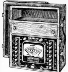
DC VOLTS: (25,000 or 1,000 Ohms per Volt); 1, 3 1/2, 7, 35, 140, 350, 700, 1400. AC VOLTS: 7, 35, 140, 350, 700, 1400. OHMS: 500, 5,000, 50,000, 500,000. 5 Meg., 50 Meg. WITH internal batteries. DC CURRENT: 0, 7, 35, 140, 350 MA; 0, 14 Amps. DECIBELS: —0 to +46. OUTPUT: 0, 7, 35, 140, 350, 700, 1400. NO CONDENSER REQUIRED. In modern steel cabinet size 9 1/16x6 3/4x5 3/8". Weight, 9 lbs. Complete with instructions and Registration Card. Regular Net Price, \$54.85.
