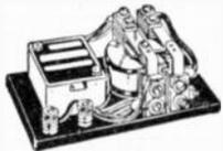
A complete 110 V. A.C. operated DPDT relay with thermostatic control for pre-heating tube filaments. Delay interval adjustable from 10 seconds to 1 minute. Relay has 1/4" silver contacts.
