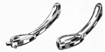
(A) 901D TURNOVER TYPE For the critical listener where true fidelity is necessary. Will track standard records at 7 grams as well as the new fine groove LP types. Knob at end of arm positions needles. Has .0027" osmium tip for standard and .001" sapphire tip for LP types. Both needles are replaceable. Output level 1-volt. Frequency to 6,000 cps. Arm is light weight curved design with single hole mounting.
