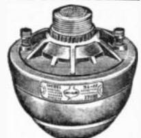
MODEL MA-25. NEW LOW-COST 25-WATT DRIVER UNIT. Similar in appearance to Illus. at right above, this new unit has ALL the fine features of "University" Drivers. Continuous service; Breakdown proof construction; Frequency Range is 90/6,000 cps. for Voice or Music work; Voice Coil Imped., 16-ohms. Size, 4½" dia.; 3¾" high. Stock No. 31B25. University Model MA-25 Driver Unit. Net. . . . \$14.70
