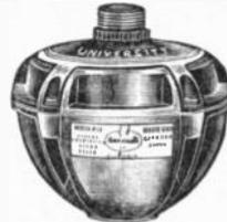
MODEL SA-HF 25-Watt Wide Frequency Range Driver Unit. Ideal for combination voice-music use due to extended frequency range of 90/10,000 cps. Will "stand up" under continuous 25-watt input; completely weatherproof; 16-Ohm V.C. Size, 4½" dia.; 4¾" high; weight, 5 lbs. A brand NEW unit scheduled for wide usage in P.A. work! (Illus. right above.) Stock No. 34B134. University Model SA-HF Driver Unit. Net. . . . \$21.76
