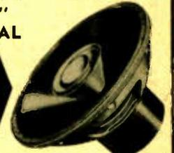
Model 102FR. Handles full 20 watts. Seamless molded curvilinear cone for lowest frequencies, and Silver Spiral differential diffuser give more extended range and greater efficiency than other single voice coils; flat within 5 db. from 50 to 9500 cps. Has powerful 4 lb. Alnico V magnet, aluminum frame. Suitable for outputs from 8 to 16 ohms. Dia. 15<sup>1/8</sup>", depth behind baffle 8<sup>1/2</sup>". Shpg. wt. 30 lbs.
