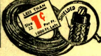
Size 22, stranded tinned copper conductor with vinylite insulation, glass braid and overall tinned copper shield. Top quality. ANJ48 specs. Ideal for phono leads and many applications where shielded hook-up wire is desired. Shpg. wt. 2 lbs. 100 ft.
