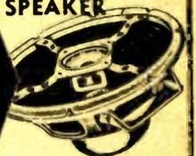
Consists of a 12-inch 6.8 oz. Alnico V PM with 1" voice coil, heavy one piece ribbed cone and coaxially suspended, 2.15 oz. Alnico V, 3" hard cone tweeter. A high pass filter is built in and concealed under pot cover. As simple to install as an ordinary PM... Only two wires to connect. Standard 8 ohm input impedance. It's the ideal speaker for the critical music lover. Response is from 40 to 17,000 cps. Shpg. wt. 8 lbs.
