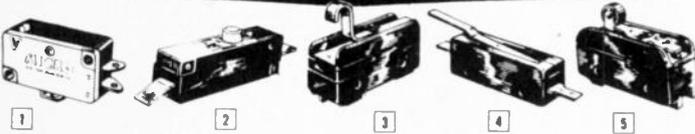
(1) Miniature Micro V-3. SPDT 10 amps @ 125 or 250 V. 1 3/8" x 7/8" x 1 3/8". Insulated plunger travels .047". O.T. .031". Wt. 2 ozs.
