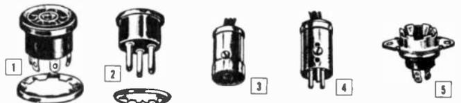
Any plug in this group mates with any socket with same number of pins. 78 series mount in 5/16" hole with push-on spring ring. Can be chassis mounted or wired to cable. 7-pin sockets fit 7-pin miniature tubes. Avg. shpg. wt. 5 ozs. per 20. Fig. ③ and ④ are 5/16" dia., 1 1/4" long cadmium plated brass. Fig. ⑤ is shielded chassis socket. Avg. shpg. wt. 1/2 ozs.
