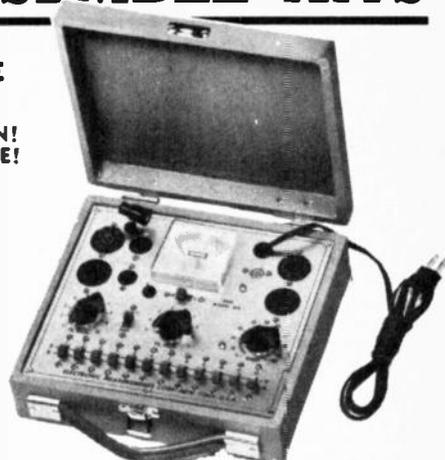
Up to date in every way. Checks all the new 12 prong (Compactron), Nu-vistor, Novar and 10 prong tubes in addition to octal, loctal, miniature and 9 prong tubes. Tests each tube for shorts, as well as for quality. Tube quality is indicated directly on a three color meter dial. Each section of a multi-purpose tube is checked separately.
