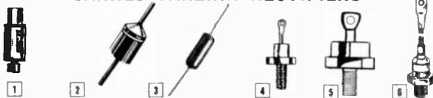
Dimensions: Fig. 1 overall 3/8" dia. x 1" L.; Fig. 2 Body .195" dia. x .335" L.; Fig. 3 Body .125" dia. x .342" L.; Fig. 4 10-32 Stud x 1.25" overall length; Fig. 5 1/4-28 stud x 1.435" overall length; Fig. 6 3/4-16 Stud x 6 1/4" overall length. P—cathode connected to stud. N—anode connected to stud.
