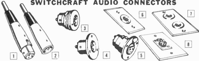
Interchangeable with Canon XLR-3, XLR-4 and Amphenol 91-850 series. Professional style audio connectors made for rugged service. Connectors are polarized with exclusive grounding lug on all units. Shells are made of die-cast zinc, satin nickel finish. Inserts are of high-impact plastic. Wall plates are brushed stainless steel and fit standard electrical outlet boxes.
