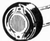
Tiny glass enclosed cell, 1/8 x 1/2" dia. Cell resistance changes with light. Operates sensitive AC relay without amplifier. Interesting and practical circuits included.
