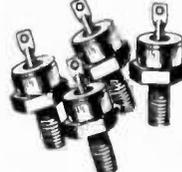
4 - 2 Amp Silicon Rectifier. Rugged stud mount. 50 PIV. rugged construction. DO-4 case. Positive polarity. 20A1120. 4 For ..... 99c
