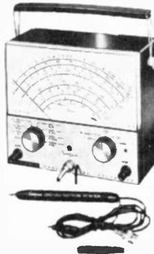
Operates for over 300 hours on a single 9 volt battery. Battery condition checked instantly. Self-shielding movement is shockproof and overload protected. All voltage range inputs are fully protected, too. Even AC line voltage can be applied on ohms ranges without damage to the Field Effect Transistor input. 7" Scale.
