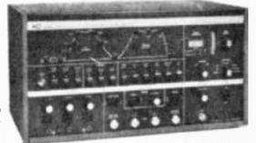
Markers are clearly indicated by lights on the panel and by tilting markers on the serviceman's scope. The unit is so complete—all that is needed to complete the alignment job is a scope and an alignment tool. Even the instruction book is different—showing a simplified, new easy method to align all TV receivers.
