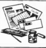
**Professional Etching Kit P101A.** An etched circuit kit utilizing photo engraving process for fine professional quality work. A negative of layout is produced, then the sensitized sheet of copper clad phenolic board is exposed through the prepared negative after which it is developed and etched. Contains three sensitized boards (2—3x6, 1—3x3), 3 mechanical negatives of the same size, etch solution, wand developer, printing frame, trays, etc. with instructions. Wt. 3 lbs.
