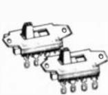
3 Pole, 3 Position Slide Switch. Control to 9 different circuits. 5/8" W. x 1 1/8" L. 3 amp, 125 V. AC. By Stack-pole.
