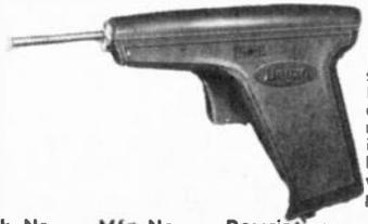
Dual heat, Hi-Lo switch in handle selects 500°F or 900°F Temperature. Lightweight... less than 5 oz. without cord set. Solid state components replace heavy transformer. Electrically isolated tip safe for soldering IC's and FET's. Solders in seconds. Complete with long chisel, short chisel and pyramid tip.
