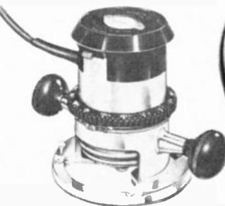
Micrometer type depth adjustment of .004". Each full turn of adjusting ring equals .004". Adjusts from 0" to 1". Depth can be changed without removing from work. Uses standard 1/4" shank tool bits. Powerful 5 amp 115 Volt AC motor has lifetime lubricated bronze and ball bearings. 20,000 rpm free spindle speed. 3 conductor cord, die-cast aluminum housing. Shpg. wt. 6 3/4 lbs.
