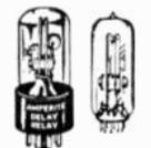
Standard type are 2 7/8" high, less pins, x 1 1/4" maximum diameter, have octal base. Miniature type are 2 1/2" above pins x 2 7/8" diameter with 9 pin miniature base.
