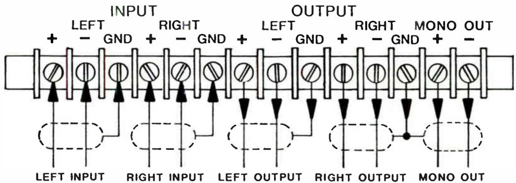
FIGURE 2-5 BALANCED LINE CONNECTIONS
