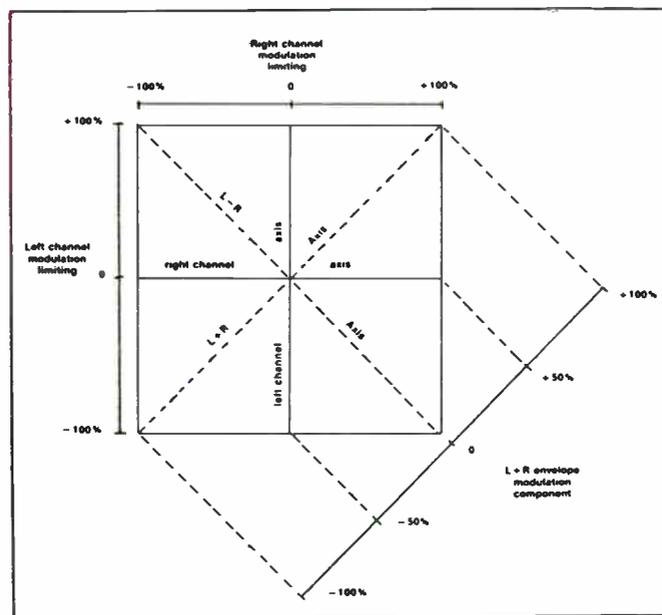
FIGURE 5-1 CONVENTIONAL STEREO LIMITING
