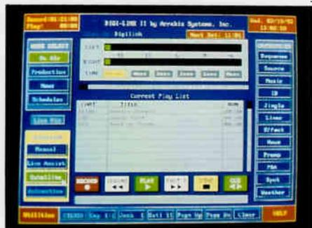
*In the 'Satellite' automation mode under 'On Air,' the system will display time to next scheduled spotset and will automatically play commercials, liners, station ID, etc.*
