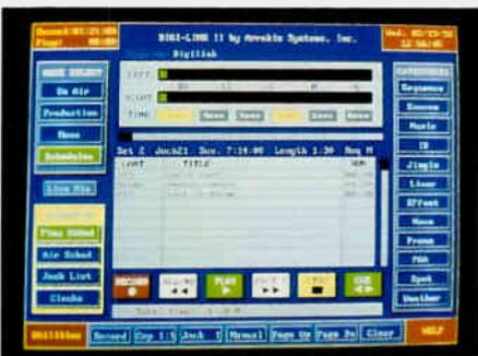
Digilink only leaves the main screen for 'Set up' or computer type 'Utility' operations. The screen at the right shows system information available under the 'Utility' button.
