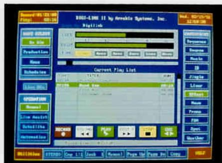
*When the 'On Air' mode is selected, either 'Manual' operation or several forms of automation may be selected. Under 'Manual,' you may play individual files or build up a sequence of files that will play back to back.*
