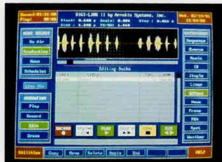
*In the 'Production' mode, 'Edit' may be selected. Under edit, multitrack mixing and reel machine type cut and splice editing are featured.*
