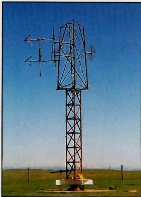
*JAMPRO also offers pattern measurement service for FM antennas at our test range. The customer's antenna is mounted in ten different positions on a tower that best simulates the actual broadcast tower, and an azimuth pattern is measured at each position. Broadcasters may then review the patterns and make an educated decision as to how their antenna should be mounted for best performance. JAMPRO stocks most types of towers, and offers tower duplication service for tower types not in stock.*
