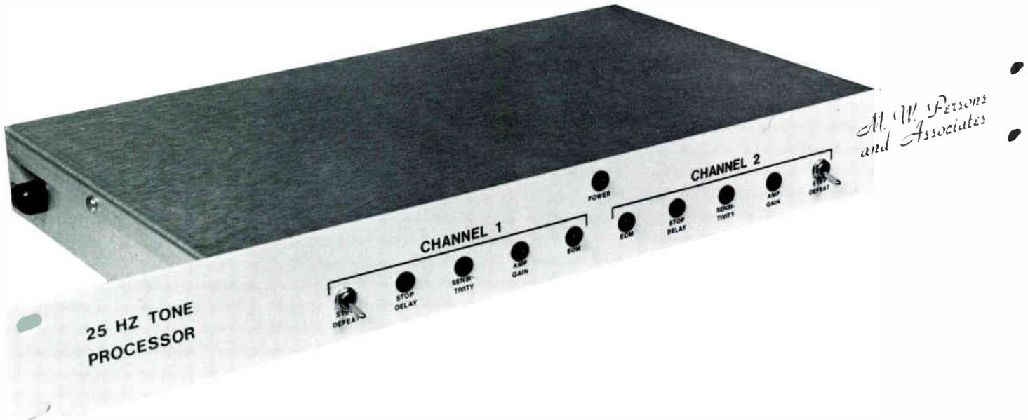
\*Dual 25Hz Tone Detectors and Dual Program Amplifiers with 25Hz Notch Filters.
