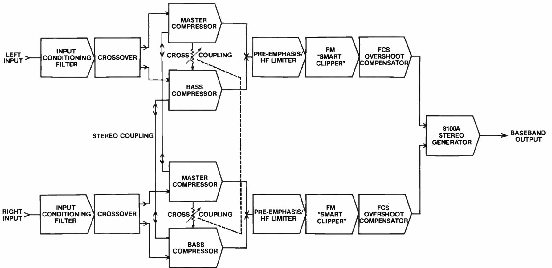
**OPTIMOD-FM MODEL 8100A SIGNAL FLOW DIAGRAM**
