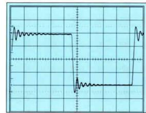
Figure 1: Typical response of uncompensated low-pass filter showing significant overshoot. (1kHz square wave)
