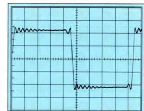
Figure 2: OPTIMOD-FM's overshoot compensated filter showing negligible overshoot. (1kHz square wave)
