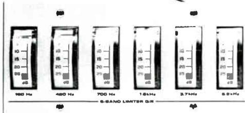
Gain reduction meters for each band: they provide the information you need for accurate setup.
