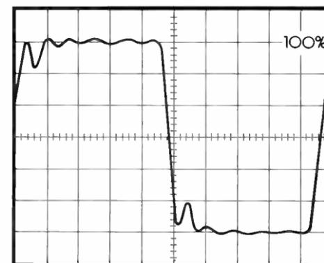
These scope photos compare the 1 kHz square wave response of the OPTIMOD lowpass filter with a conventional stereo generator's lowpass filter. Ringing in the conventional unit forces the steady state level down to 70% modulation to avoid overmodulation - a loudness loss of 3.1 dB compared to OPTIMOD.
