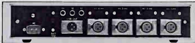
Rear view of RA-4 Remote Amplifier showing terminals.
