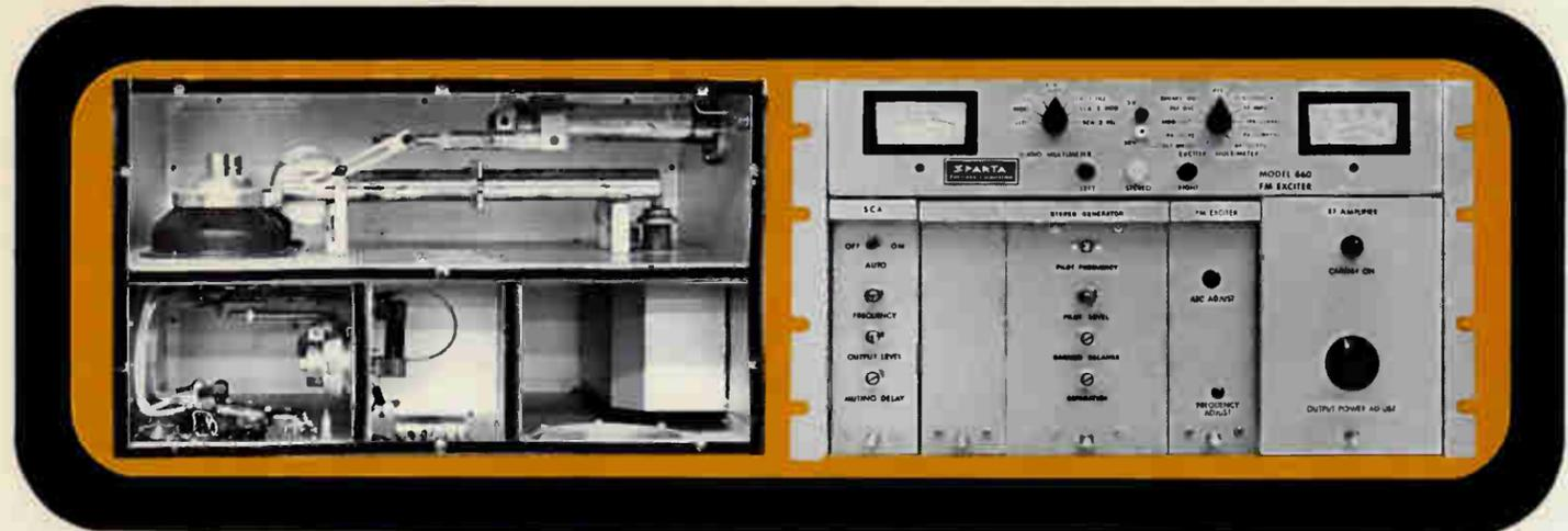
The heart of the Model 603A-5 FM Transmitter is the Model 660 FM Exciter, shown above right. An all solid-state unit providing monaural, stereo and/or SCA modes of operation. The 660 Exciter allows 5 to 15 watts output power into a matched 50 ohm load. The modulation method is "direct carrier FM" with no mixers or multipliers after the modulated oscillator. Maintenance of the
