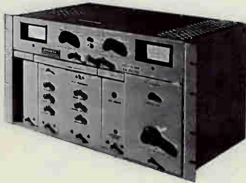
**MODEL 660.** The Model 660 is the solid-state heart of every SPARTA FM transmitter. It is shown (right) complete with its plug-in stereo and SCA modules. Its rating is 10 watt direct carrier FM, although its full capability is up to 15 watts. Alternate uses are for educational FM broadcasting, or FM band STL.
