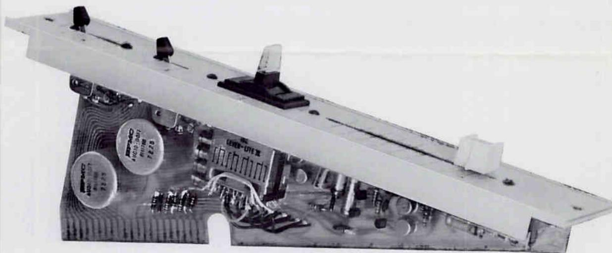
The modern, modular design of UREI's Mod One broadcast consoles provides a wide choice of plug-in input modules to meet specific requirements in AM and FM broadcasting. All modules mate automatically in any of the 10 module positions of the MOH-110 or MOH-210 consoles, allowing optional organization of console functions with minimum installation labor. Blank modules may be installed in unused positions, and used for custom controls, etc., or future expansion.
