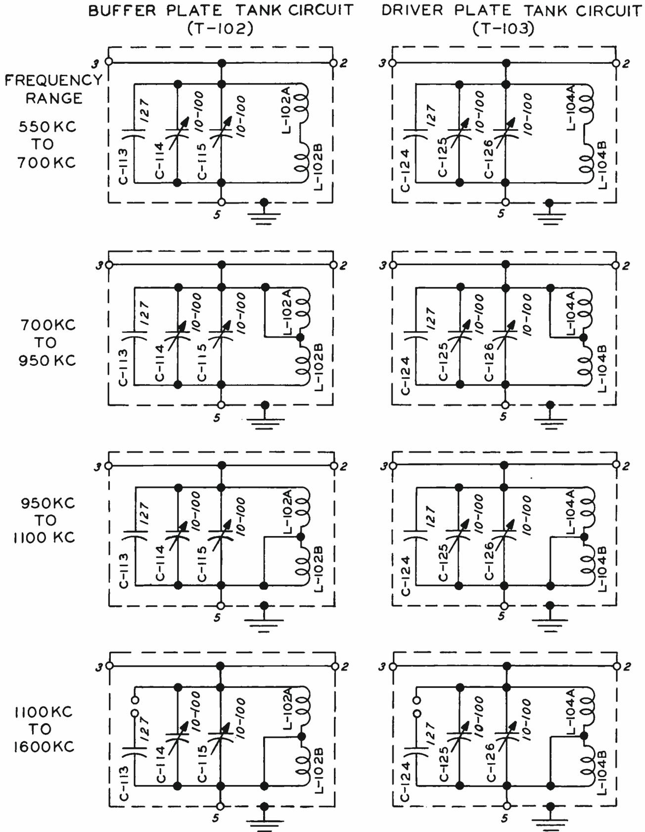
Figure 7-2. T-102 and T-103 Internal Connections
