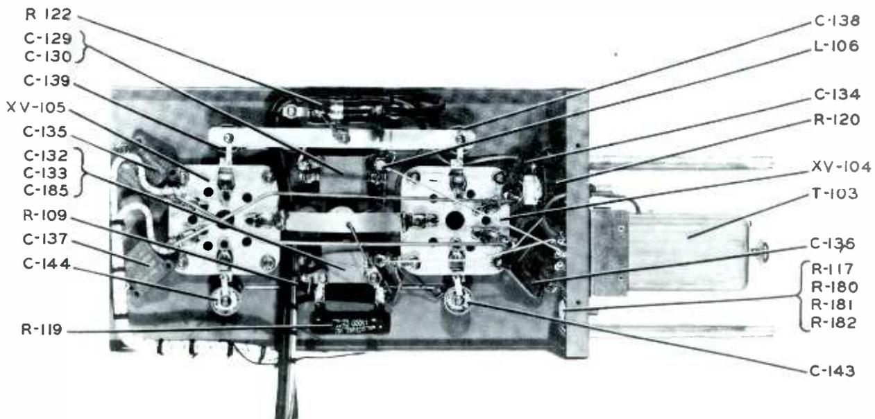
Figure 6-4. R-F Chassis Parts Arrangement, Bottom View
