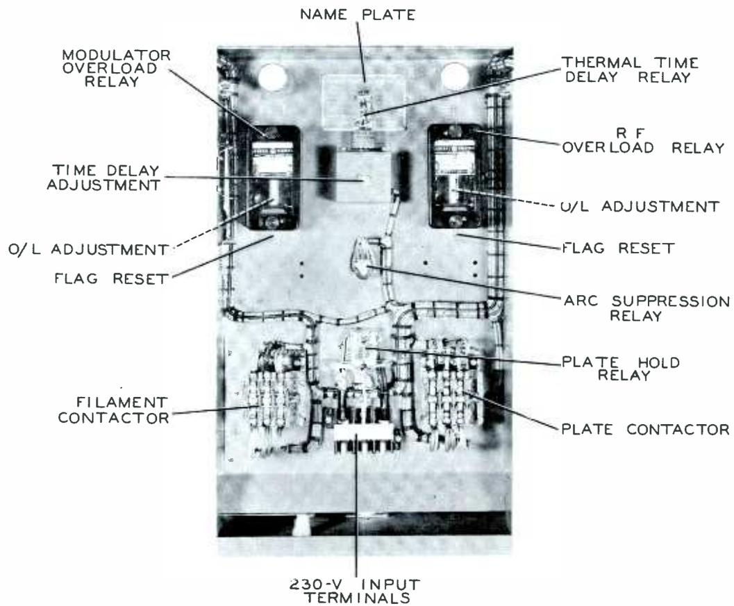
Figure 6-10. Relay Panel Controls
