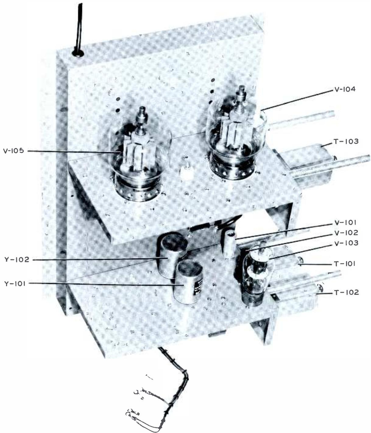
Figure 6-3. R-F Chassis Parts Arrangement, Top View
