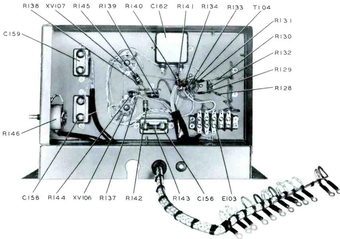
Figure 6-6. Audio Chassis Parts Arrangement, Bottom View
