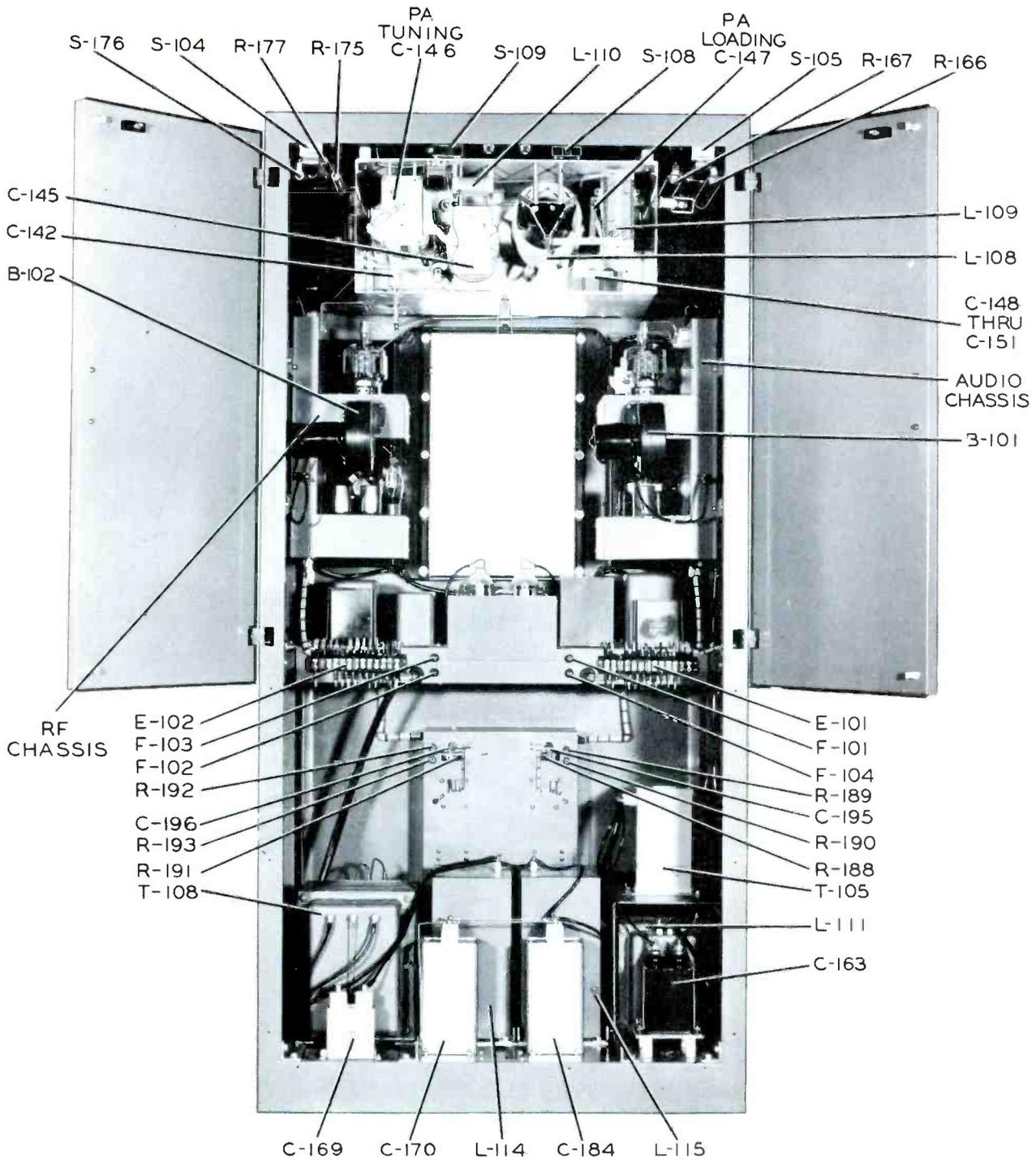
Figure 6-2. Transmitter Parts Arrangement, Rear View
