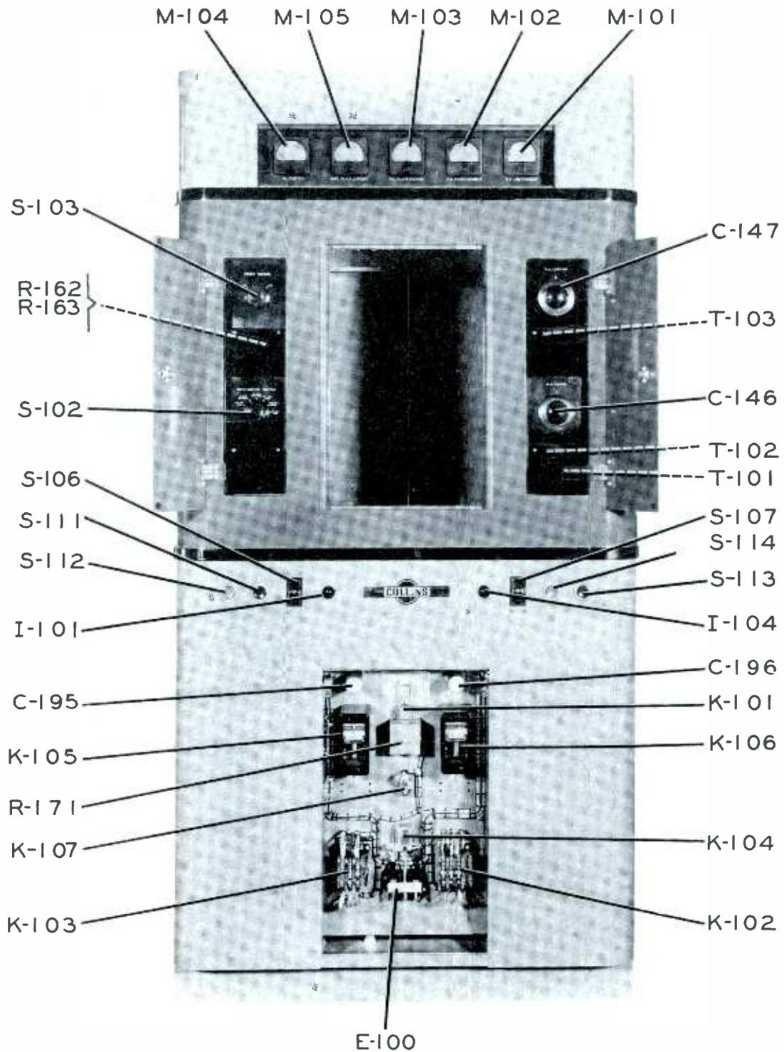
Figure 6-1. Transmitter Parts Arrangement, Front View
