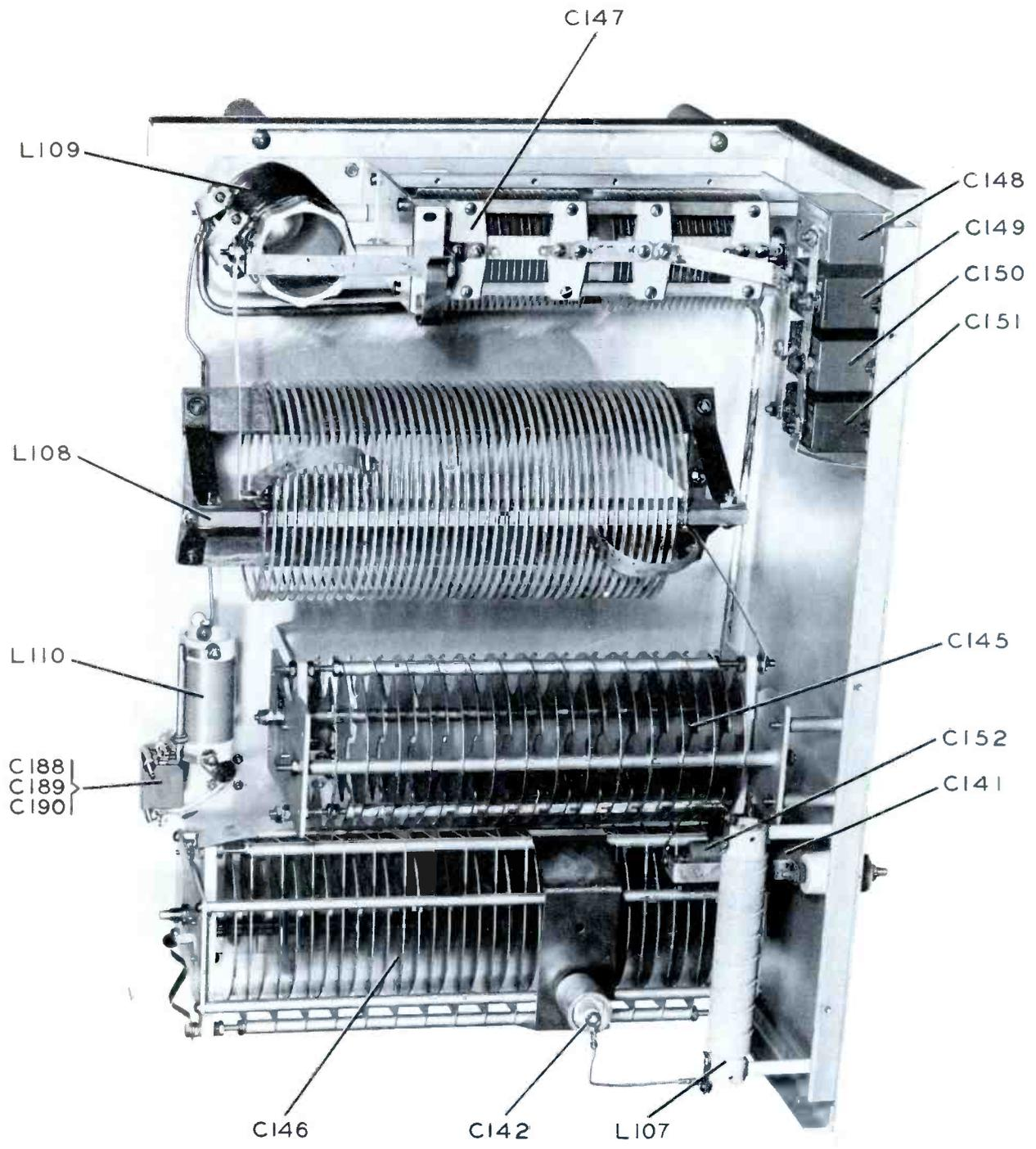
Figure 6-7. Output Network Parts Arrangement, Bottom View
