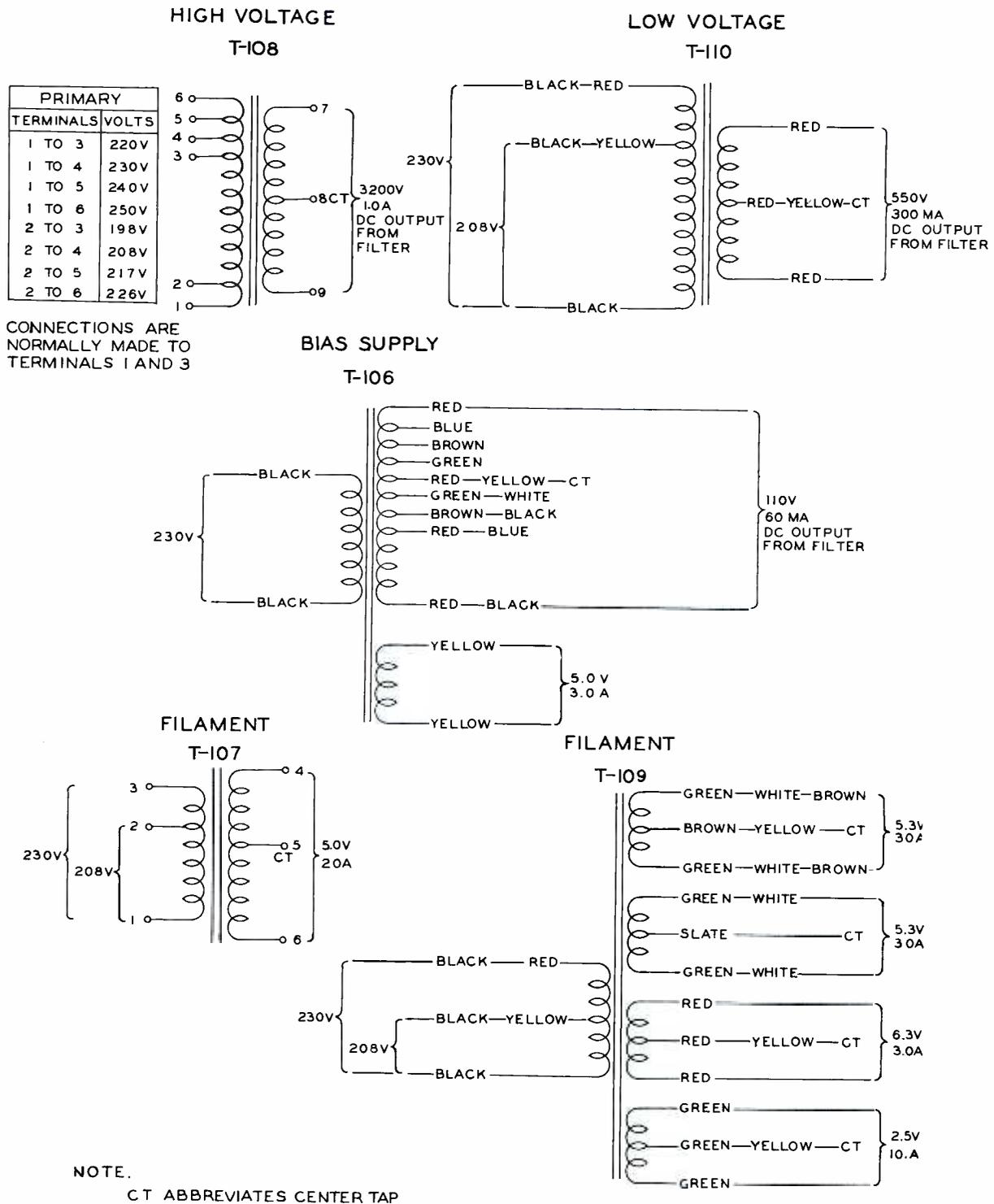
Figure 7-4. Transformer Details
