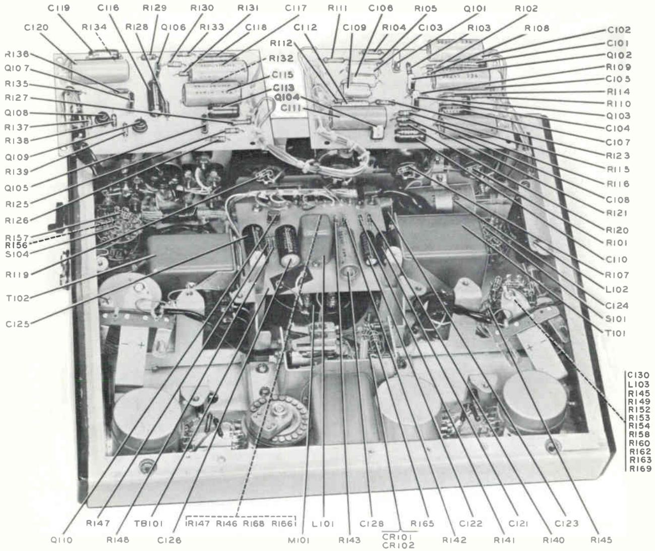
Figure 7-2. 212Z-1 Remote Amplifier, Bottom Open, Boards Removed
