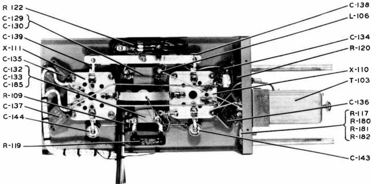
Figure 7-9. Driver Cabinet RF Chassis, Bottom View.
