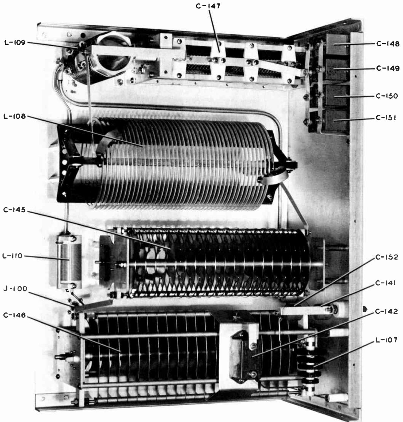
Figure 7-13. Driver Cabinet Output Network, Bottom View.
