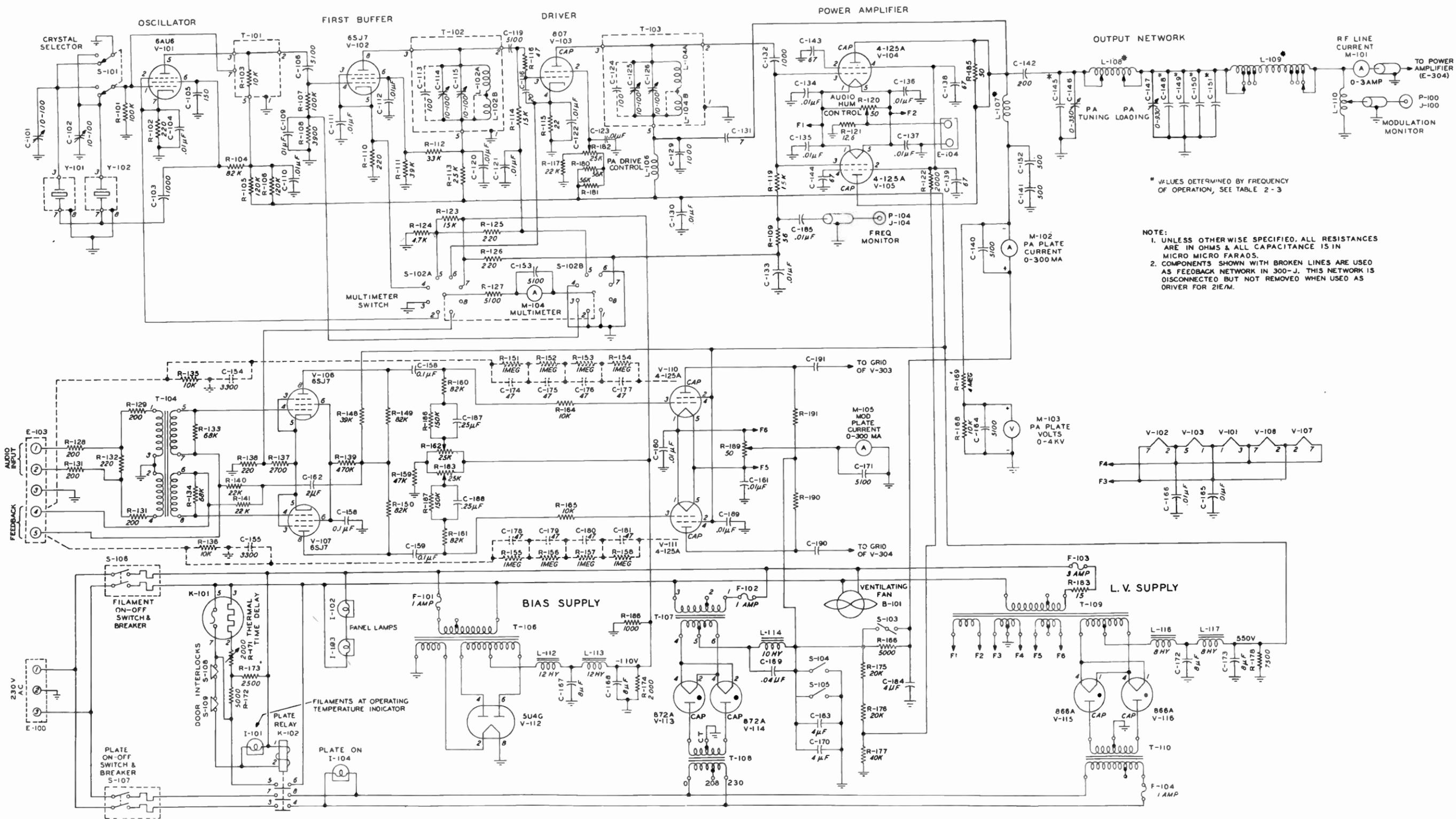
Figure 8-2. Driver Cabinet Complete Schematic.
