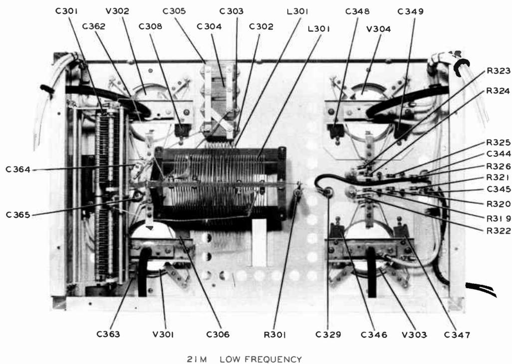
Figure 7-5B. Power Amplifier RF Chassis, Bottom View
