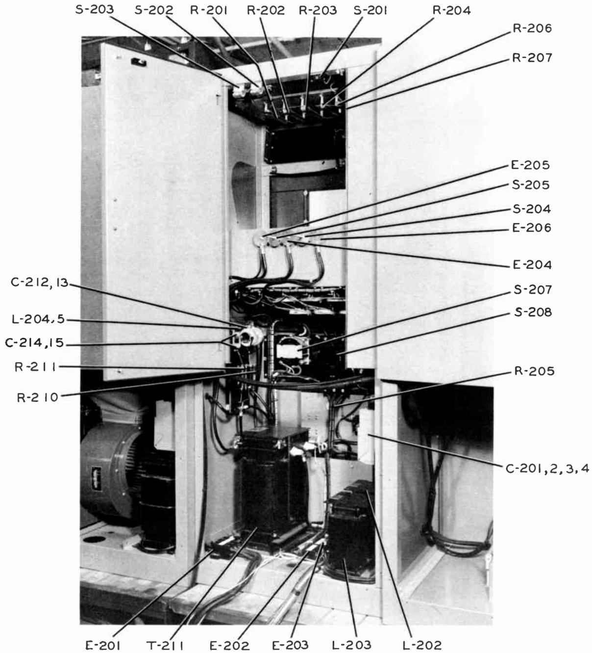
Figure 7-2A. Power Supply Cabinet, Rear View.
