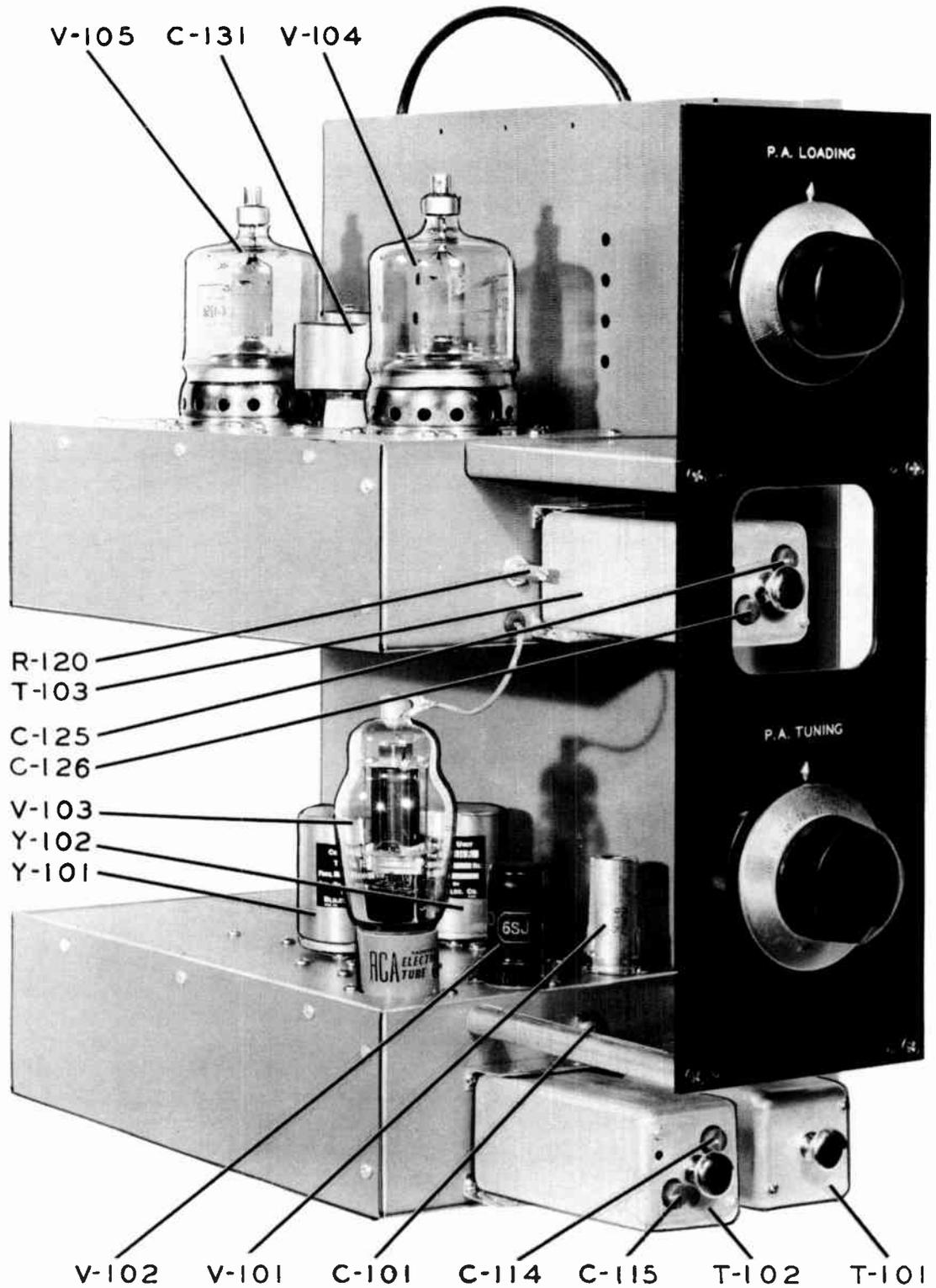
Figure 7-8. Driver Cabinet RF Chassis, Top View.
