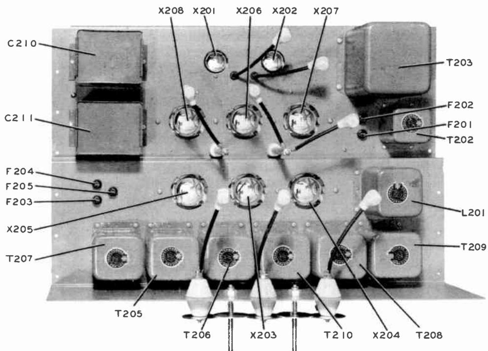
Figure 7-6. Power Supply Cabinet Rectifier Chassis, Top View.
