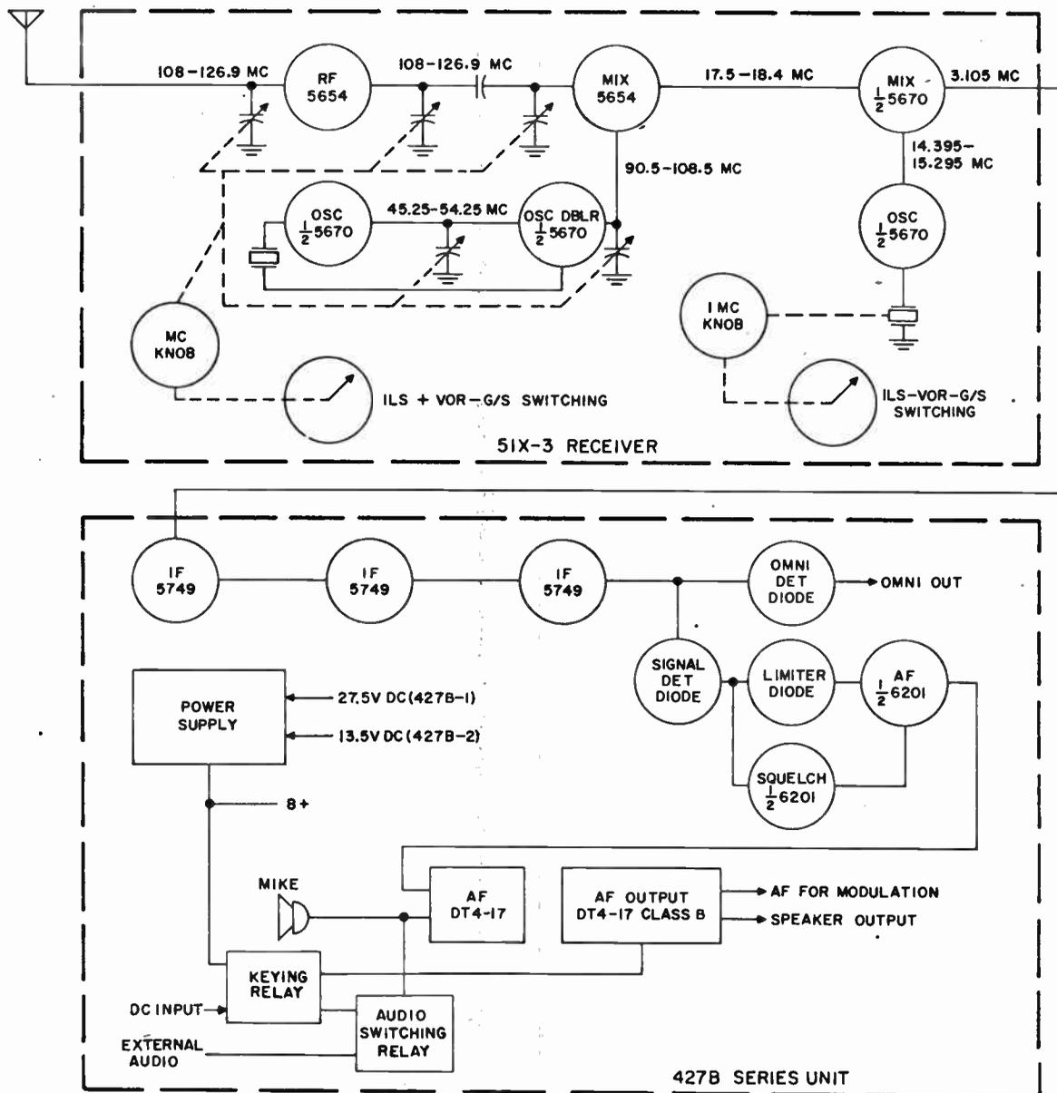
Figure 4-1. Receiver 51X-3 and 427B-( ) Unit, Block Diagram
