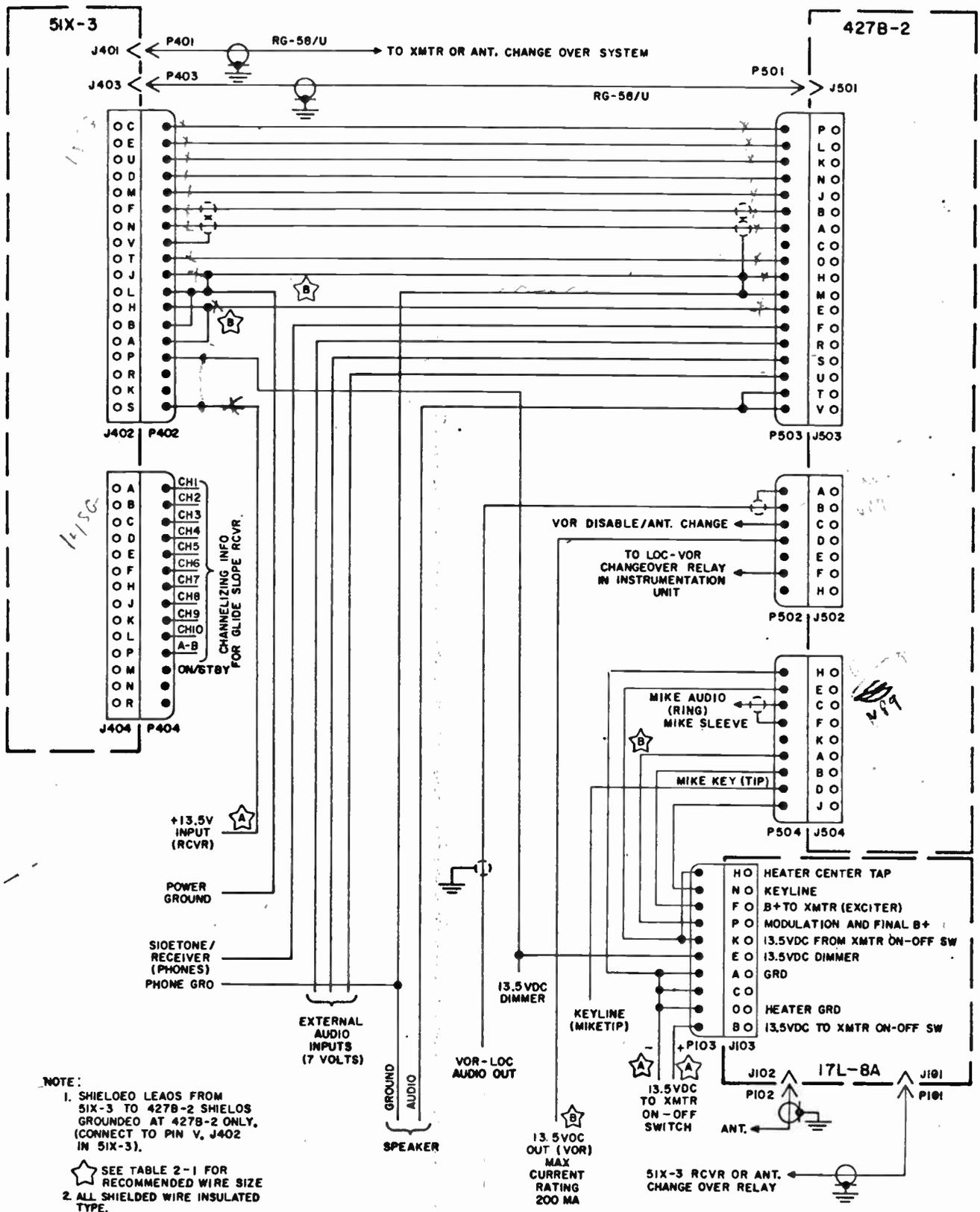
Figure 2-4. 51X-3, 427B-2, 17L-8A Interconnecting Cabling Diagram
