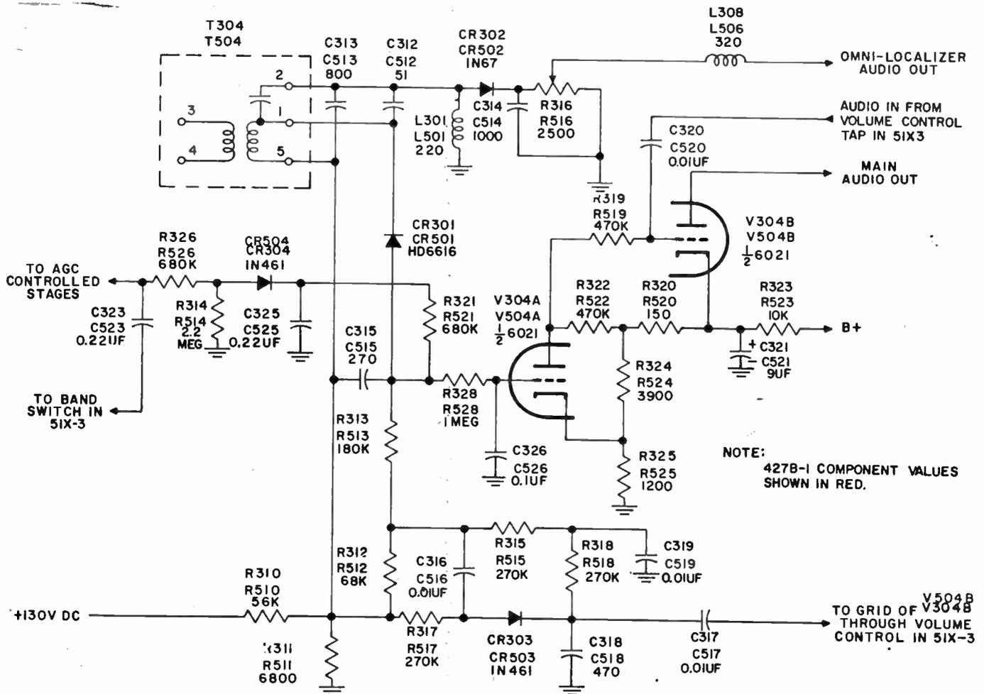
Figure 4-2. Detectors, AGC, Squelch and Noise Limiter Circuits, Schematic Diagram
