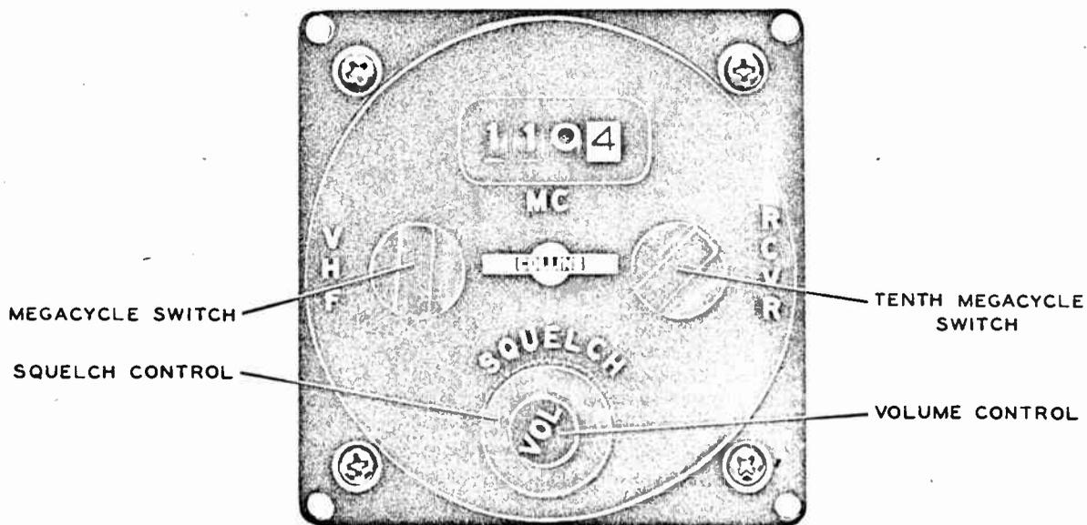
Figure 3-1. Receiver 51X-3, Operating Controls
