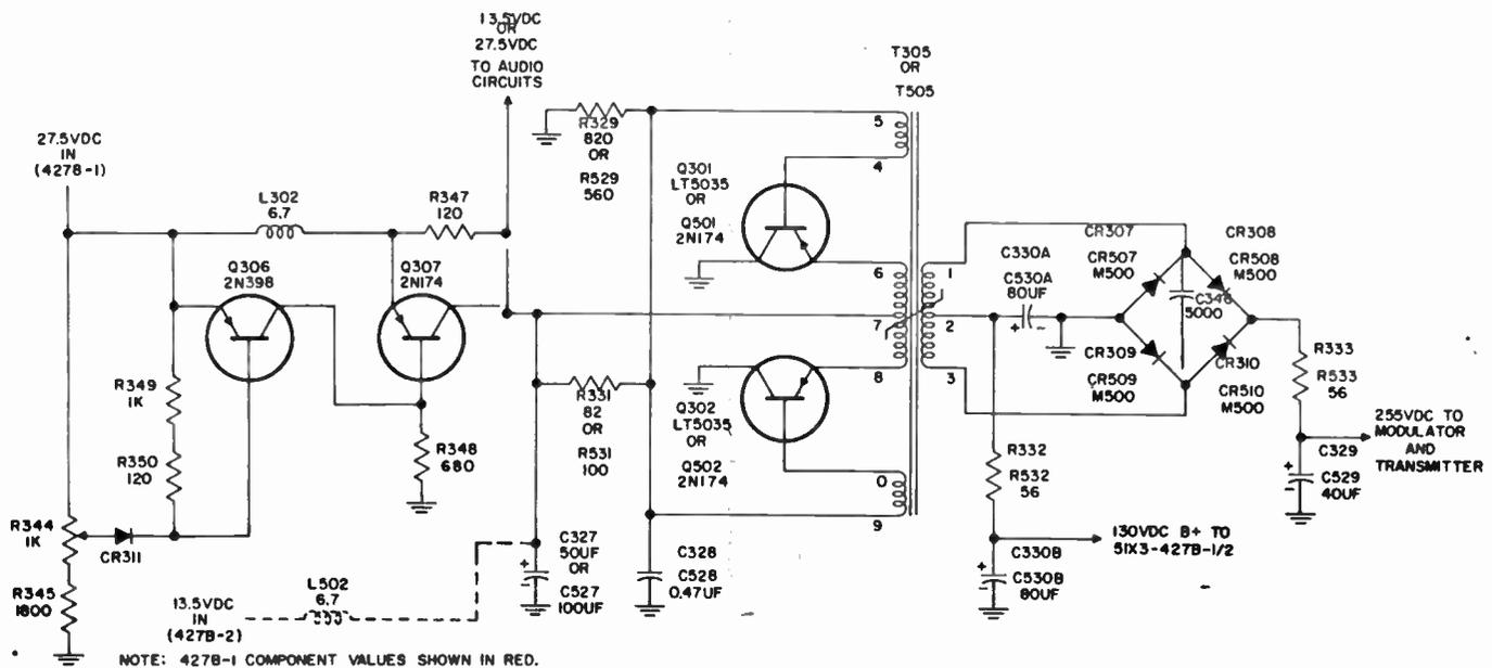
Figure 4-3. Power Supply, Schematic Diagram
