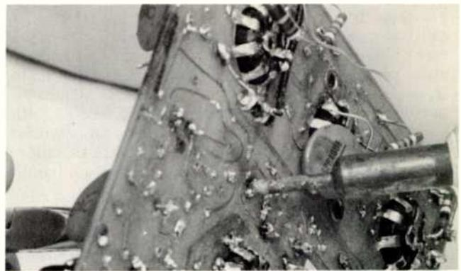
Figure 6-6. Push Leads Out Component Side of Board
