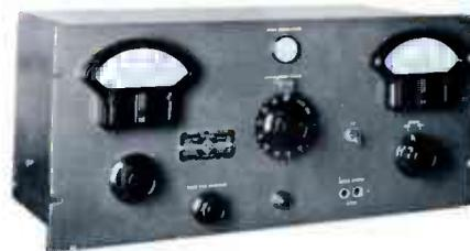
Operating in the frequency range of 0.5 to 8 mc, the 1931-A measures percentage modulation on either positive or negative peaks, indicates over-modulation, monitors program level, measures carrier shift when modulation is applied and measures transmitter audio frequency response. *Size: 19"W, 8 3/4"H, 10"D, for rack mounting. Power Source: 105-125 v ac, 50/60 cps, 50 w.*
