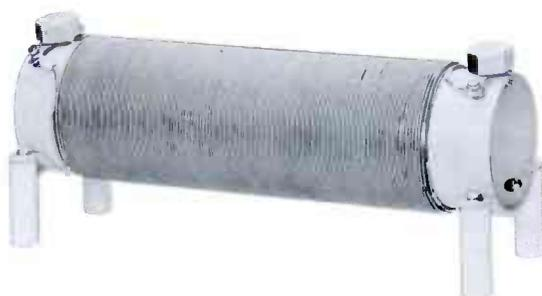
These solenoid wound 2 and 3 wire chokes provide high impedance throughout the broadcast band for isolation of the ac power lines from the antenna. Coils are wound of #10 wire and are rated at 2,000 w, 120 v ac, single phase, assemblies and provided with mounting brackets and standoff insulators for mounting in 42E-7/8 antenna coupling units. Weatherproof cabinets are available for outdoor mounting.
