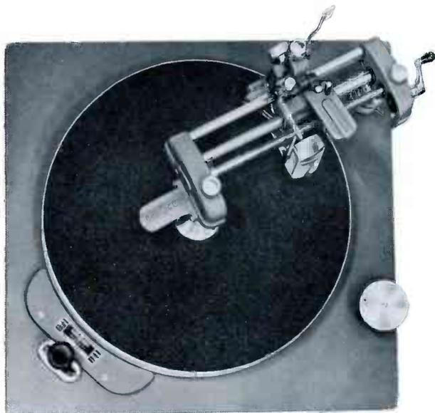
R-16H with M-5S Overhead Lathe
