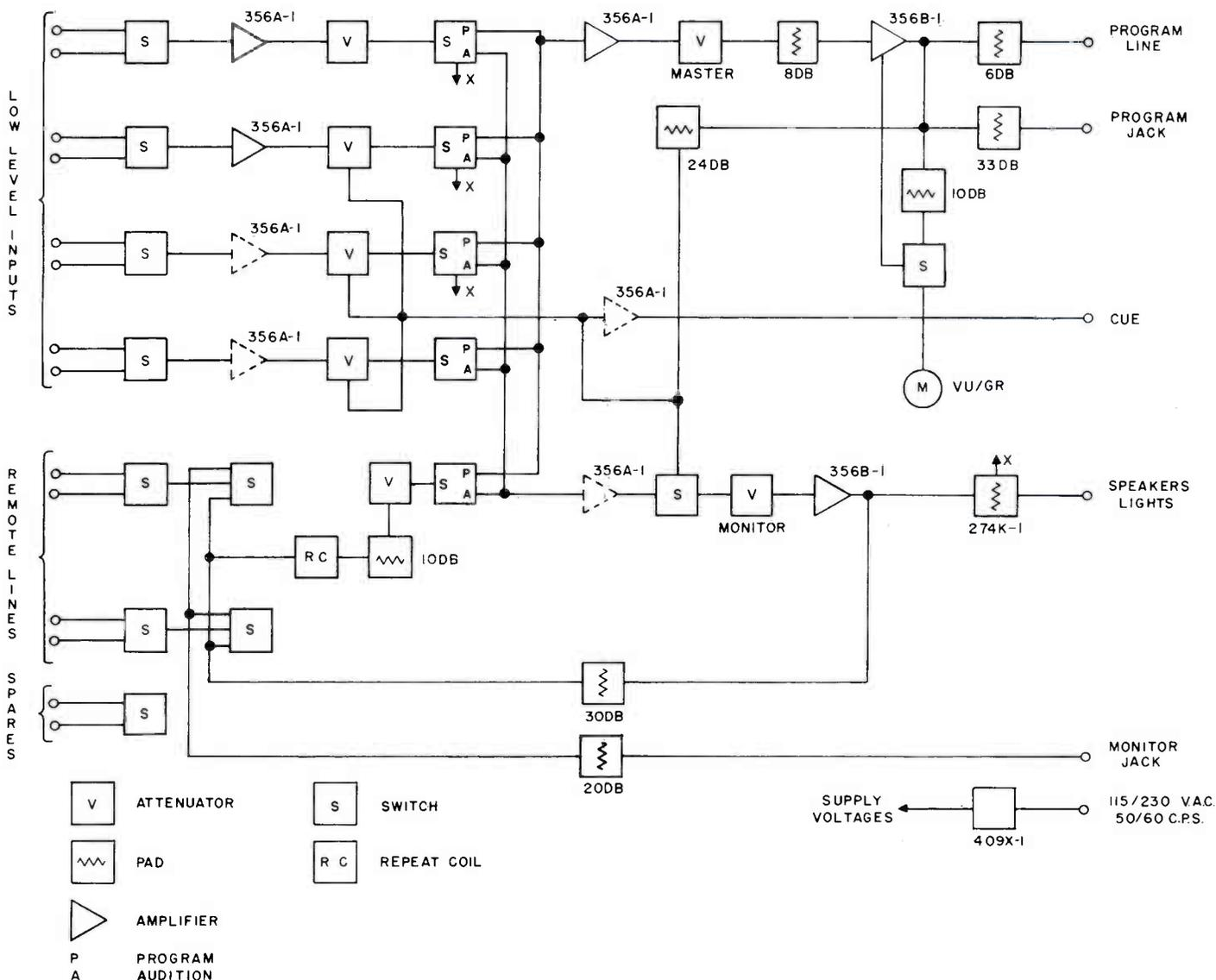
*Number of Channels:* Two low level inputs with provision for four low level input channels with the addition of two more 356A-1 Pre-amplifiers. One remote input, one program output and four monitor outputs. Cueing output from three of the low level mixer attenuators.
