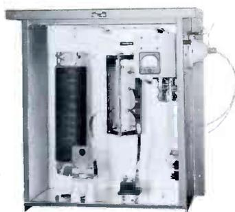
These are specially constructed units for matching a series-fed vertical radiator to an unbalanced transmission line. The electrical circuit is a low-pass T network with good harmonic attenuating properties. A three-wire or two-wire tower lighting filter choke and remote antenna current
