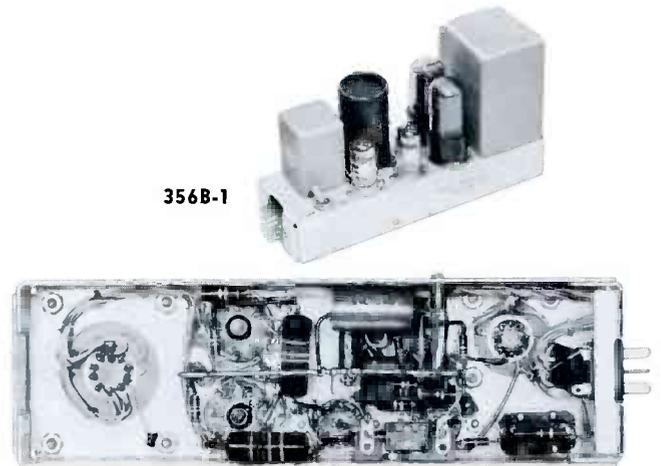
nal. *Output Impedance:* 150 or 600 ohms balanced or unbalanced. *Output Level:* +18 dbm maximum *Gain:* 40 db. *Frequency Response:*  $\pm 1$  db, 50 to 15,000 cps. *Distortion:* 0.5% maximum. *Noise:* -118 at input, or 96 db below full output. *Tubes:* 2 — 5879. *Power Requirements:* 6.3 v ac or dc at 0.3 amps. 250 v dc at 6.5 ma or 300 v dc at 7.5 ma. *Size:* 4 $\frac{5}{8}$ "H, 2 $\frac{1}{8}$ "W, 9 $\frac{1}{2}$ "D. *Weight:* 2 $\frac{1}{4}$  lbs.
