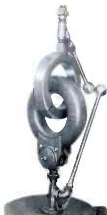
These air insulated lighting transformers are designed to produce high RF impedance to ground when used to feed ac lighting energy across the base insulator of a radio tower. Transformers can be mounted either horizontally or vertically and are available in 1.75, 3, and 5 kva sizes.
