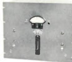
The 1181-A gives direct indication of magnitude and direction of the frequency deviation of an AM transmitter. The monitor input is obtained from the transmitter output. Positive indication of either transmitter carrier or monitor crystal oscillator is provided. *Frequency Range:* .5 to 2.0 mc. *Crystal:* Specify frequency on purchase order. *Deviation Range:* ±30 cps. *Size:* 19"W, 15 3/4"H, 13"D, for rack mounting. *Power Source:* 105-125 or 210-250 v ac, 50/60 cps 125 w.
