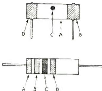
Fig. 1 — Color coding of fixed composition resistors. The color code is given in Table 1. The colored areas have the following significance:
