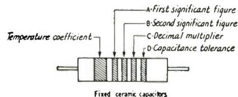
Fig. 2 — Color coding of fixed mica, molded paper, and tubular ceramic condensers. The color code for mica and molded paper condensers is given in Table 1. Table 2 gives the color code for tubular ceramic condensers.
