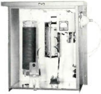
These are specially constructed units for matching a series-fed vertical radiator to an unbalanced transmission line. The electrical circuit is a low-pass T network with good harmonic attenuating properties. A three-wire or two-wire tower lightning filter choke and remote antenna current
