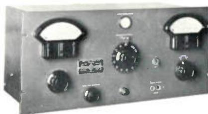
Operating in the frequency range of 0.5 to 8 mc, the 1931-A measures percentage modulation on either positive or negative peaks, indicates over-modulation, monitors program level, measures carrier shift when modulation is applied and measures transmitter audio frequency response. *Size:* 19"W, 8 3/4"H, 10"D, for rack mounting. *Power Source:* 105-125 v ac, 50/60 cps, 50 w.
