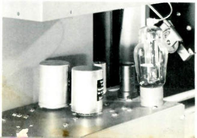
Only seven different tube types are used, resulting in fewer spares to meet FCC requirements.
