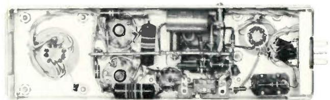
nal. **Output Impedance:** 150 or 600 ohms balanced or unbalanced. **Output Level:** +18 dbm maximum **Gain:** 40 db. **Frequency Response:**  $\pm 1$  db, 50 to 15,000 cps. **Distortion:** 0.5% maximum. **Noise:** -118 at input, or 96 db below full output. **Tubes:** 2 — 5879. **Power Requirements:** 6.3 v ac or dc at 0.3 amps. 250 v dc at 6.5 ma or 300 v dc at 7.5 ma. **Size:** 4 $\frac{5}{8}$ "H, 2 $\frac{1}{8}$ "W, 9 $\frac{1}{2}$ "D. **Weight:** 2 $\frac{1}{4}$  lbs.
