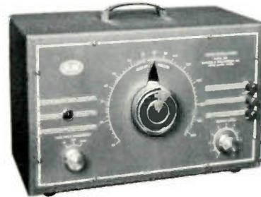
The model 200 is a resistance capacitance type for making frequency response, distortion and other audio measurements. *Ranges:* 30-300, 300-3,000, 3,000-30,000 cps. *Output:* 10 v into 500 ohm load. Less than 1% rms harmonics 30-15,000 cps with 500 ohm load. *Response:* Better than  $\pm 1$  db 30-15,000 cps. *Calibration Accuracy:* 3% of scale reading. *Size:* 13 $\frac{3}{4}$ " x 7 $\frac{1}{4}$ " x 9 $\frac{1}{2}$ ". For operation from 105-125 v ac 50/60 cps. *Shipping Weight:* 17 lbs.
